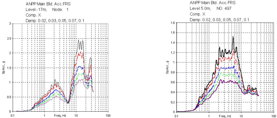
**Figure 9: Floor Response Spectra in the ANPP Main Building (courtesy Mr. P. Zadoyan, private communication)**
