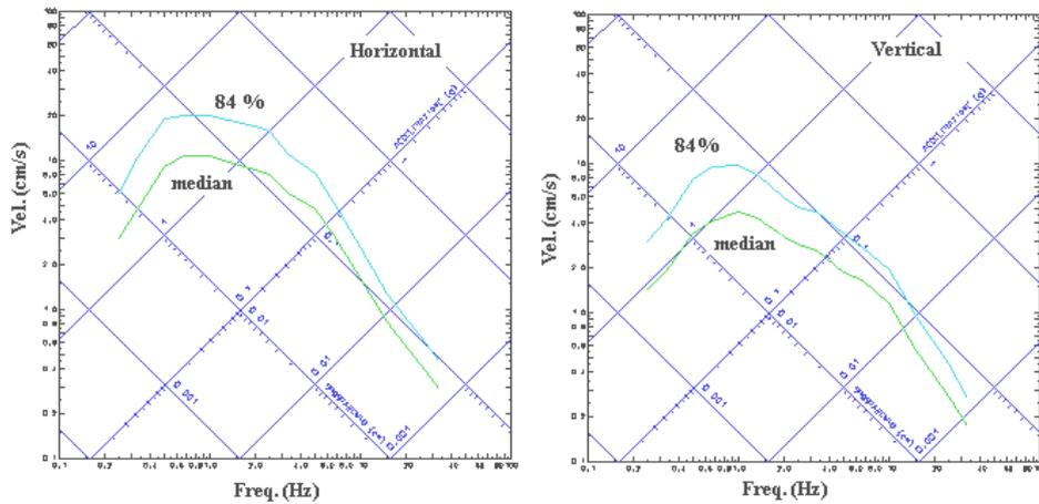
**Figure 6: Earthquake Spectra at ANPP from just the 1988 Spitak Earthquake and Sabetta-Pugliese Attenuation Law**
