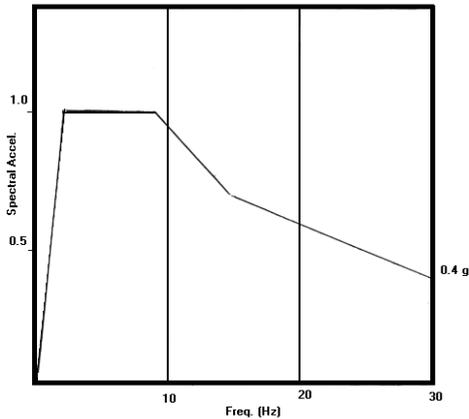
**Figure 2: Original ANPP Design Spectrum**
