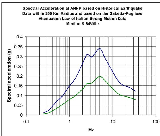
**Figure 5: Generated Spectra at ANPP from Seismic**
