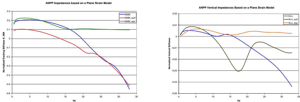
**Figure 8: Impedance Functions (real part) for Rocking and Vertical ANPP Foundation Motions**
