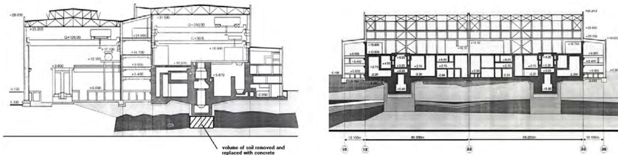
**Figure 1: Armenian NPP Cross Sections Including Details of Soil/Structure Interface**
