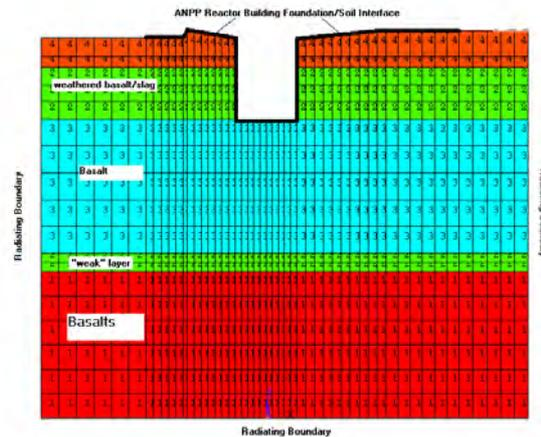
**Figure 7: Detailed FE Model of ANPP Foundation/Soil Interface and Subsurface for Impedance Calculations**
