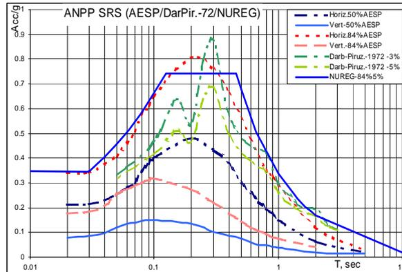
**Figure 3: Estimated Free-field Response Spectra at ANPP**
