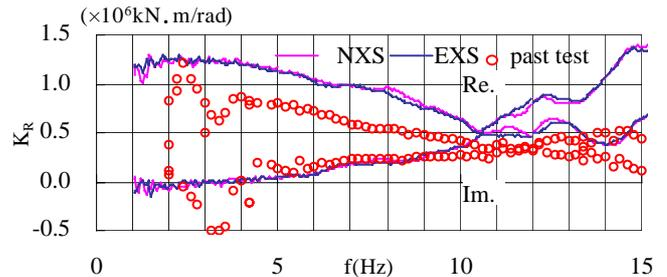
Fig. 11 Comparison of rocking spring by TEST20 and TEST21
