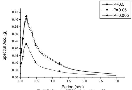
Fig. 6: 5% Damping UHRS for Various Values of P
