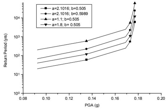
Fig. 4: Sensitivity of the Return Period for PGA to a and b (for line sources)
