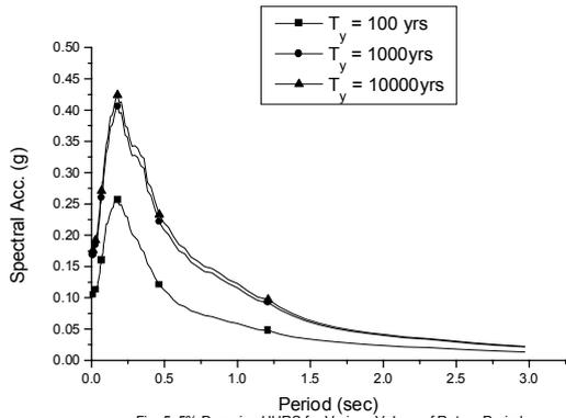
Fig. 5: 5% Damping UHRS for Various Values of Return Period
