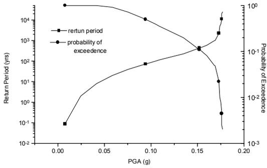
Fig.3 : Return Period and Probability of Exceedence for PGA; a= 2.1016 and b=0.5989 for Line Source
