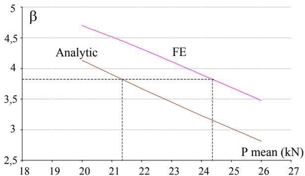
Figure 6. Comparison between analytical and finite element limit state function.
