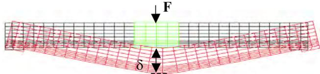
Figure 5. Deformed mesh of the beam.
