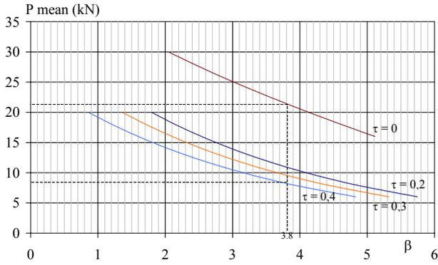
Figure 8. Reliability assessment curves of a corroded beam, analytical simulation ( $C\tau=25\%$ ,  $C_p=15\%$ ).
