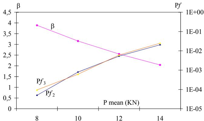
Figure 7. Comparison between level-2 ( $P_{f2}$ ) and level-3 ( $P_{f3}$ ) methods with conditioning procedure for a corroded beam.
