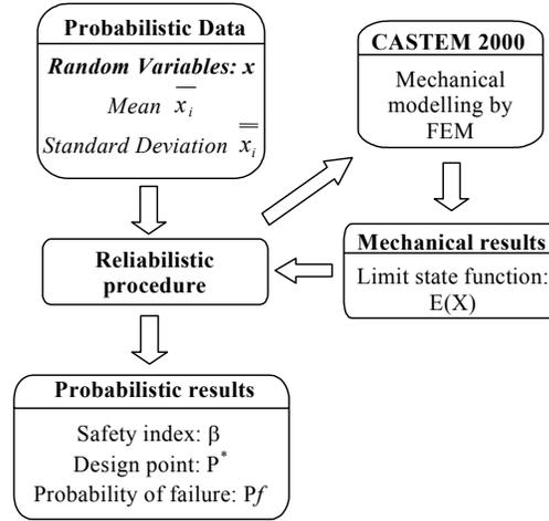
Figure 2. Coupling reliability finite element simulations.
