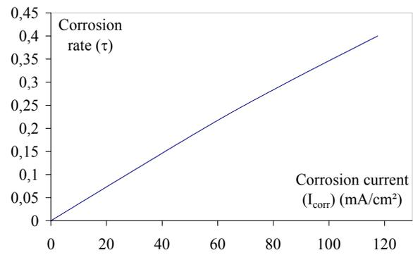
Figure 11. Corrosion rate versus corrosion current.
