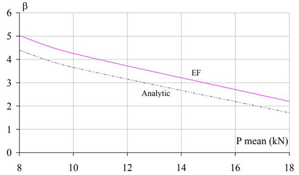
Figure 9. Comparison between analytical and finite element simulations for a corrosion rate of 20%.
