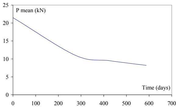
Figure 12. Evolution of carrying capacity of the corroded beam with time for  $b=3.8$ .
