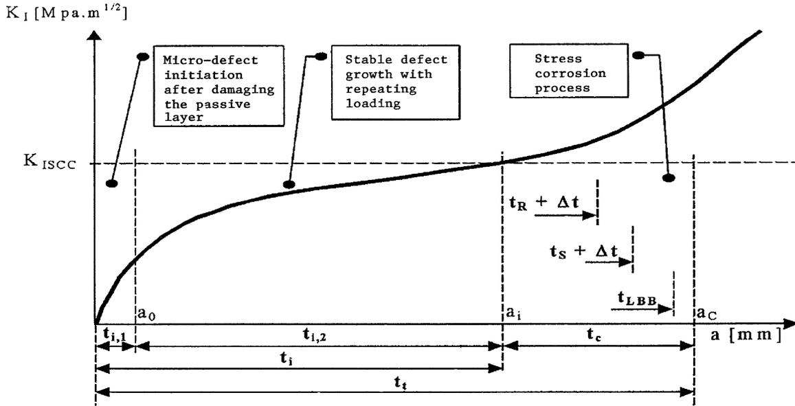
**Figure 2** The process of material degradation under stress corrosion cracking
