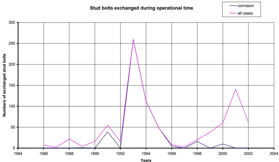
**Figure 3** Influence of used measures on decreasing number of stud bolts exchanged for corrosion damage
