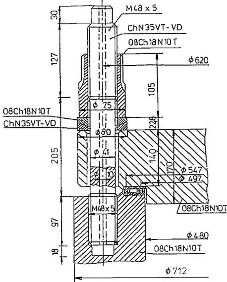
**Figure 1** Scheme of the analyzed demountable joint
