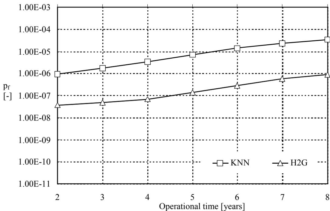
**Figure 4** Probability of the loss of cover functionality vs. service time
