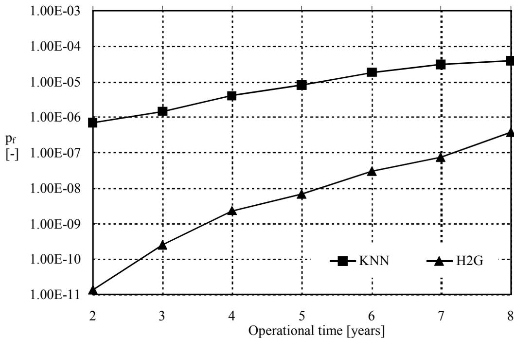
**Figure 5** Probability of first stud bolt breaking vs. service time
