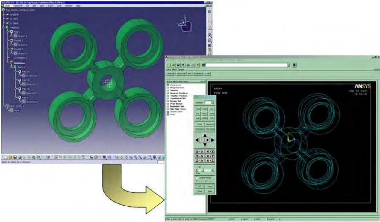
Figure 1. Direct Import from CAD System Model to Structural Analysis Tool
