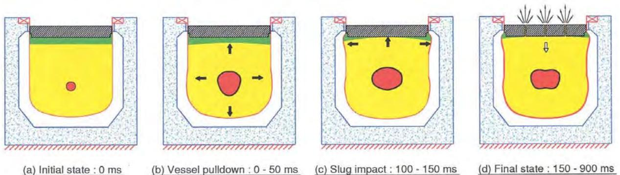
Fig.1 Mechanical consequences of CDA
