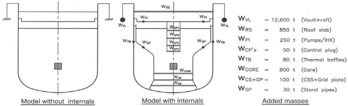
Fig.4 Idealised models used for CDA analysis
