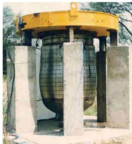
Fig.10 Deformed MV (1200 MJ case)
