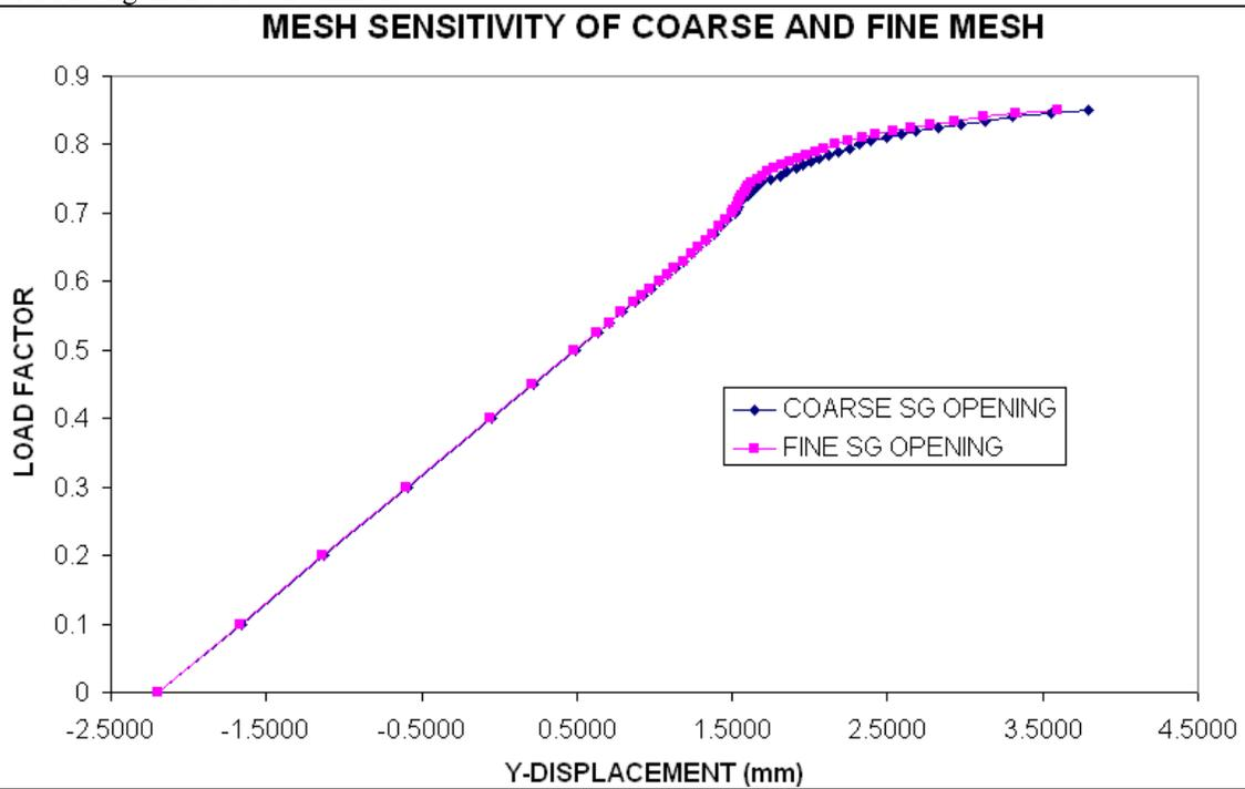
Fig.-2: Load-deformation curve of Crown and near SG opening for Mesh Sensitivity Study
