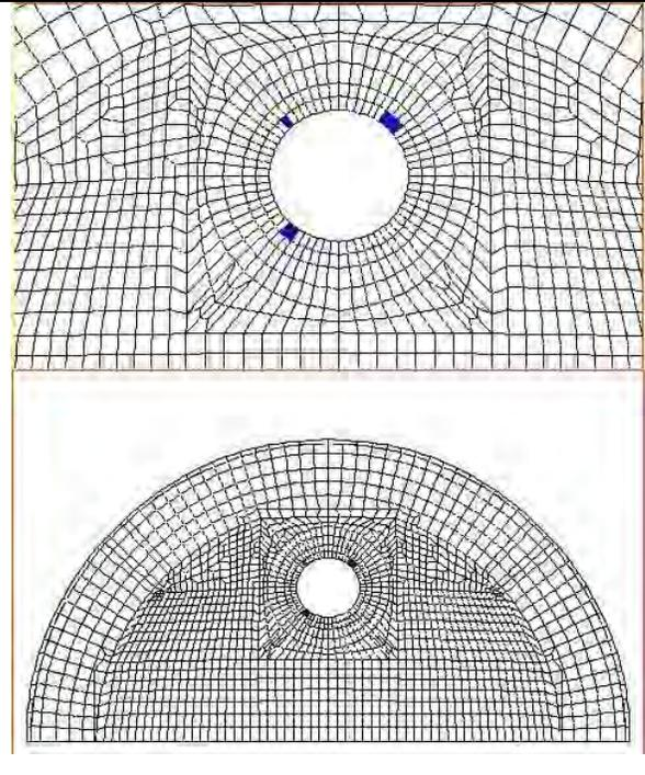
Fig.-4: Initiation of thru\_n\_thru' crack (at Load Factor = 1.4) with Accident Temperature
