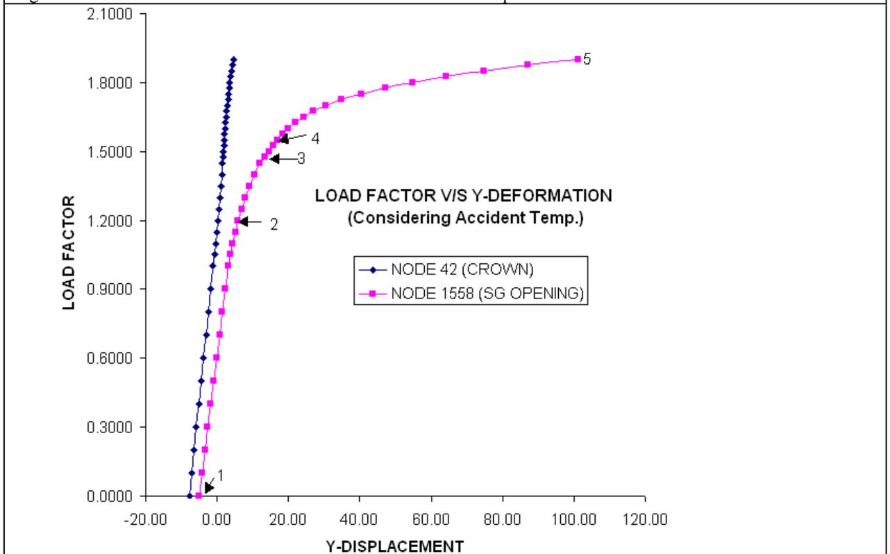
Fig.-8: Load-deformation curve of the ICS with Accident Temperature
