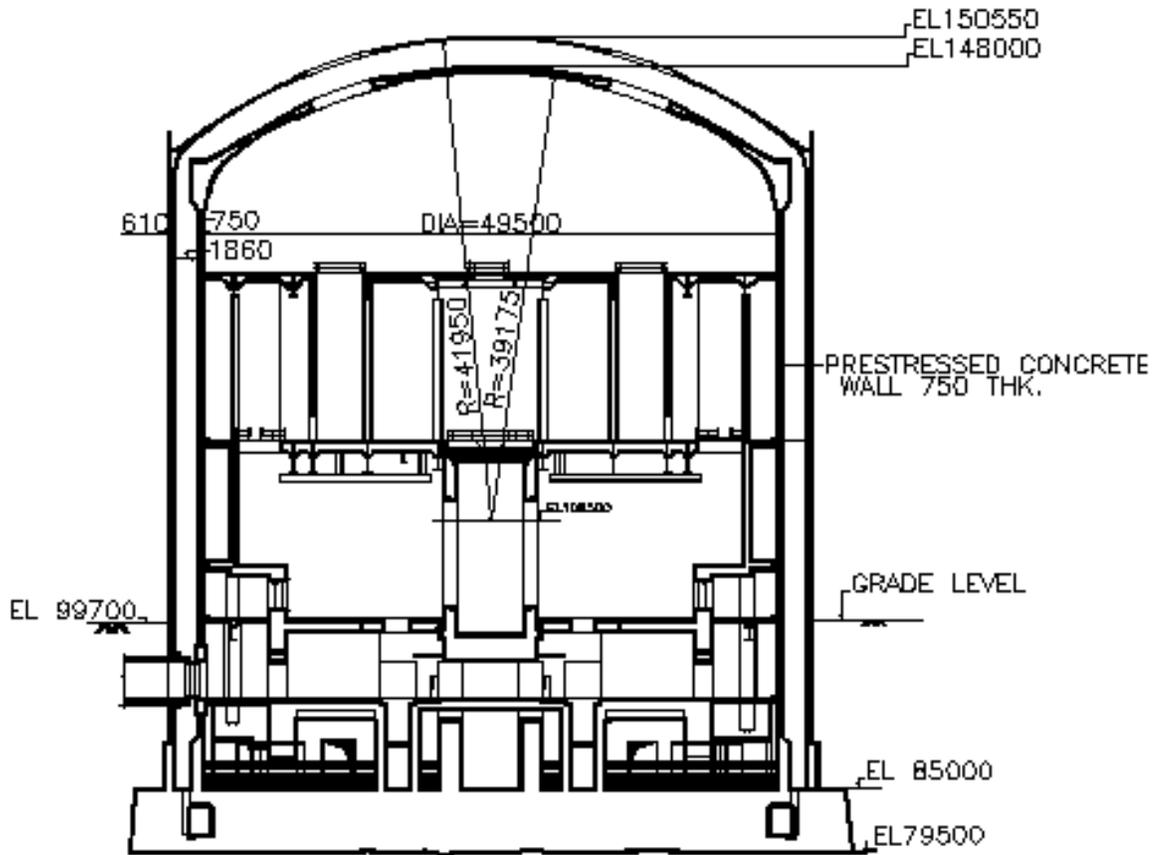
Fig.-1 : General Arrangement of Containment
