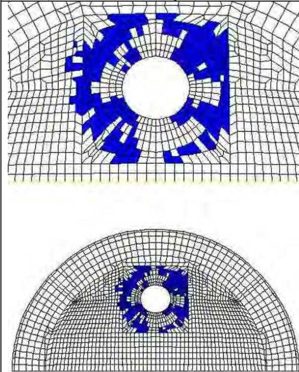
Fig.-5: Extent of thru\_n\_thru' crack at failure (at Load Factor = 2.08) without Accident Temperature
