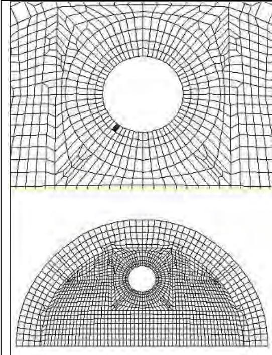
Fig.-3: Initiation of thru\_n\_thru' crack (at Load Factor = 1.425) without Accident Temp
