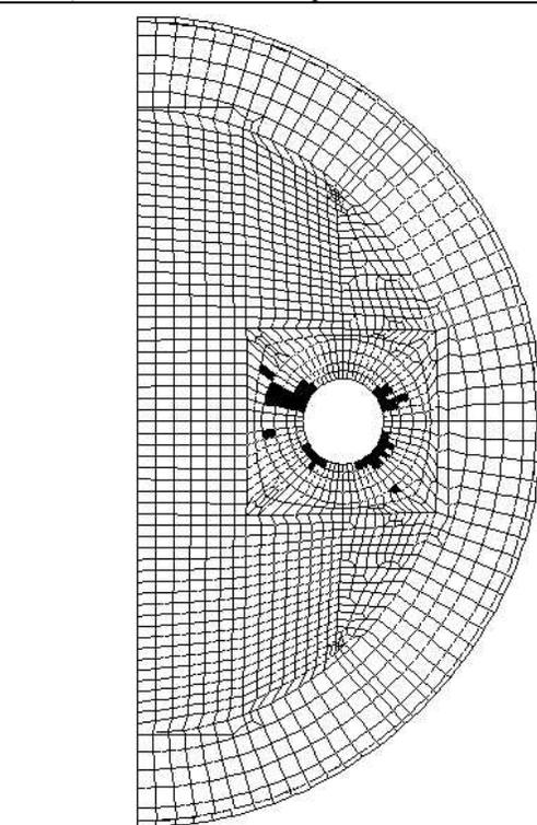
Fig.-6: Extent of thru\_n\_thru' crack at failure (at Load Factor = 1.9) with Accident Temperature
