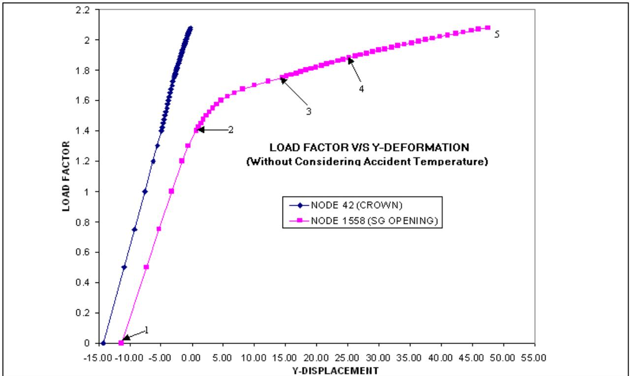
Fig.-7: Load-deformation curve of the ICS without Accident Temperature
