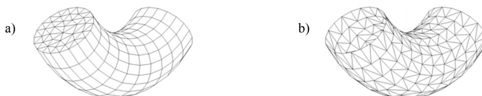
Fig. 3. Fluid (a) and pipe (b) 3D finite element meshes of the elbow zone.
