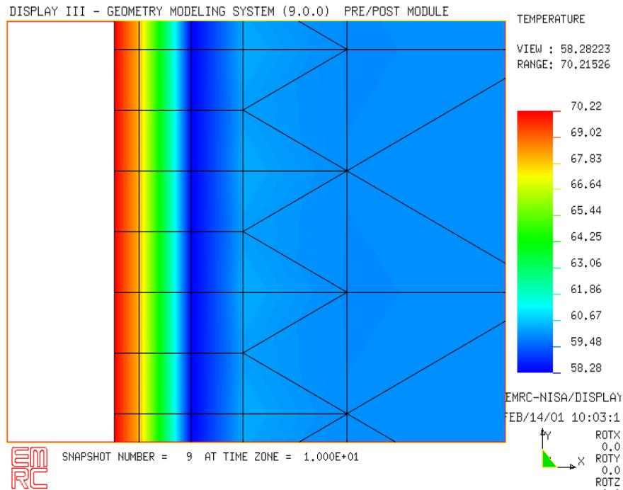
Fig. 3 Temperature distribution in the wall at 10 sec after accident
