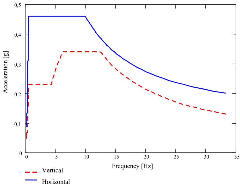
Fig.1 SL2 Free-Field Response Spectra
