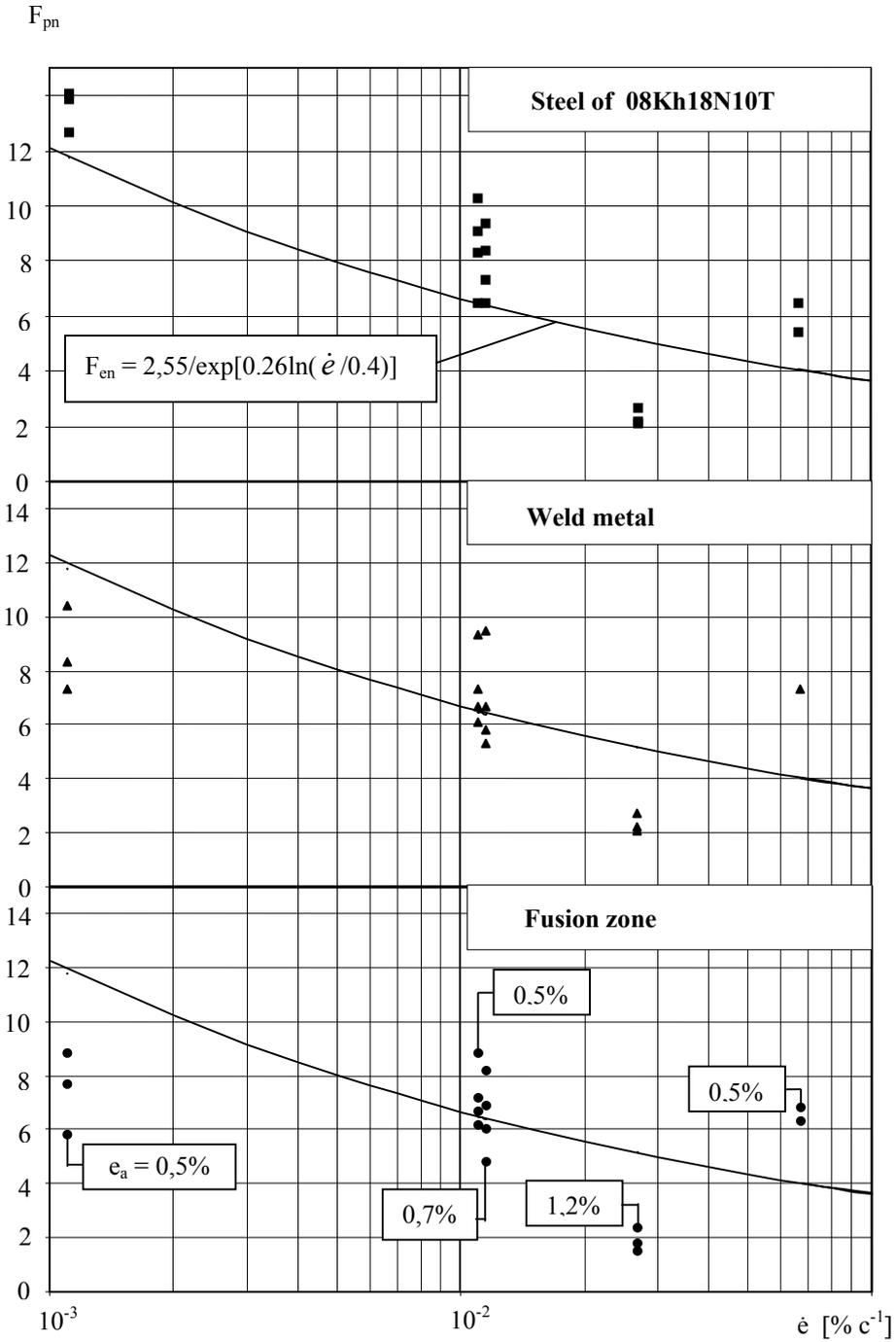
Fig. 1.  $F_{en}$  factors for some zones of 08Kh18N10T steel welded joints
