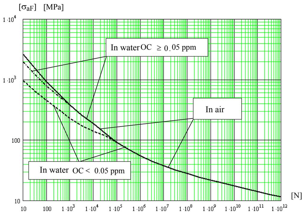
Fig. 3. Design fatigue curves for austenitic stainless steels
