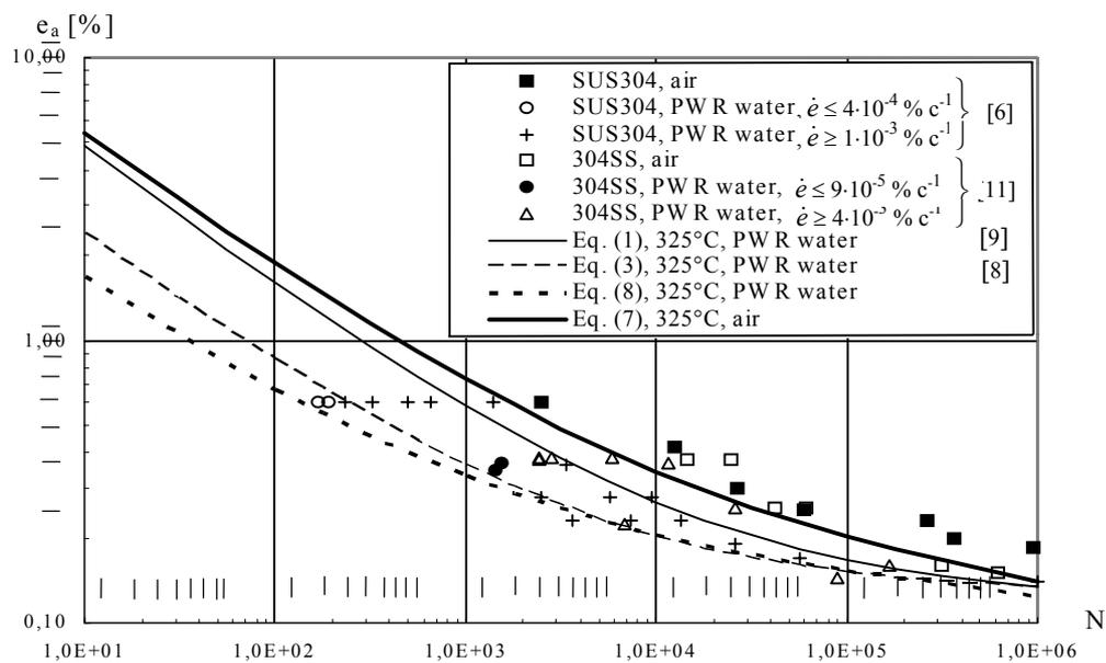
Fig. 2. Comparison of experimental results and calculated SSs fatigue curves (the strain-controlled symmetrical cycle)
