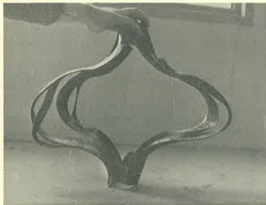
Fig. 7 - Test No. 1 - Exagonal box after the explosion
