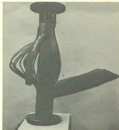
Fig. 9 - Test No. 5 - Rupture of exagonal box and test section after the explosion
