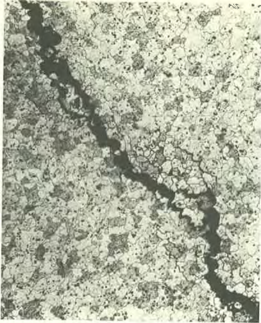
Fig. 1. Photomicrograph of Stress Corrosion Cracking in 2024-T4 Aluminum Alloy
