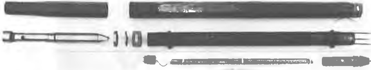
Figure 3 Exploded View of Central Sub-assembly and charge
