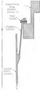
Fig. 1: The system of supporting structure
