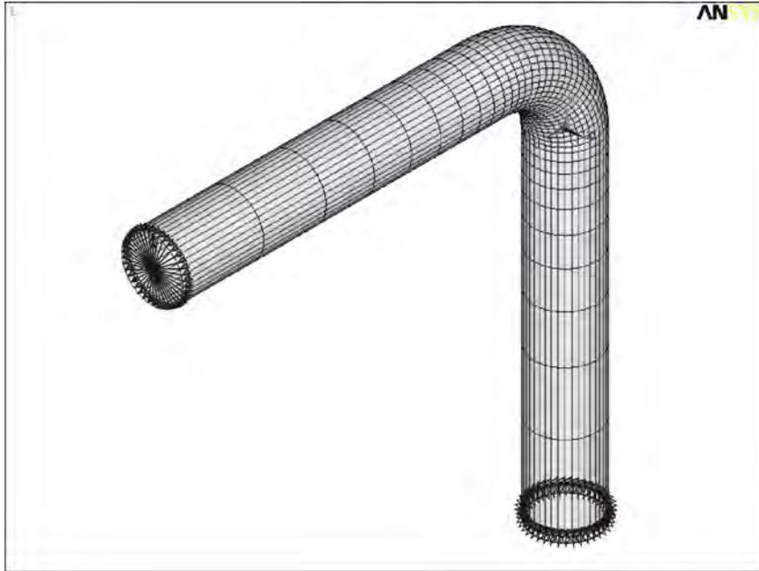
Figure 5: FEA model used for straight-pipe/bends analysis
