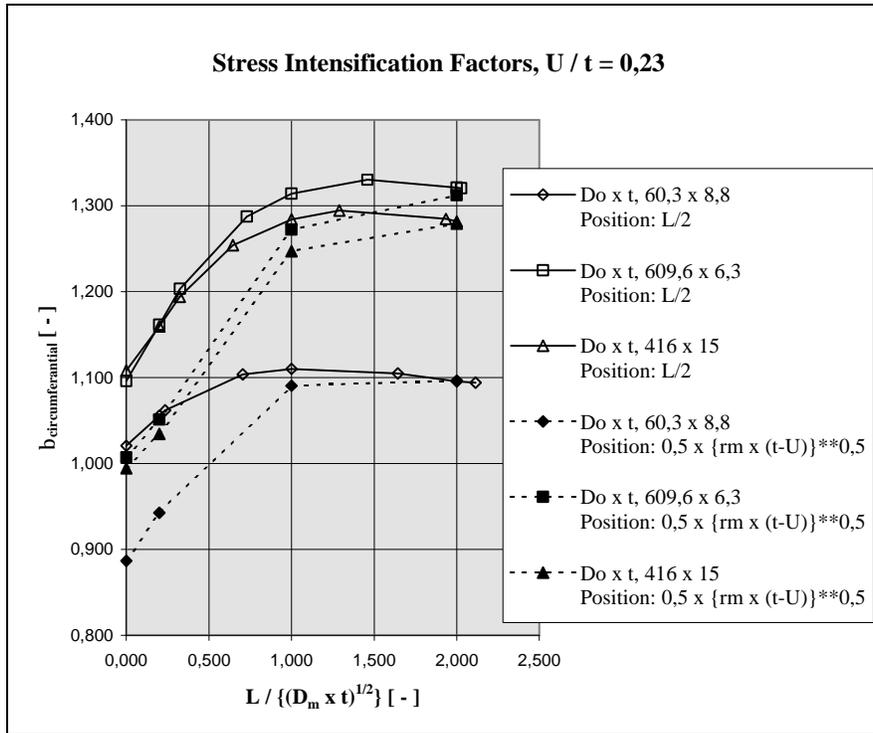
Figure 3: Circumferential SIFs, Internal Pressure,  $U/t=0,23$
