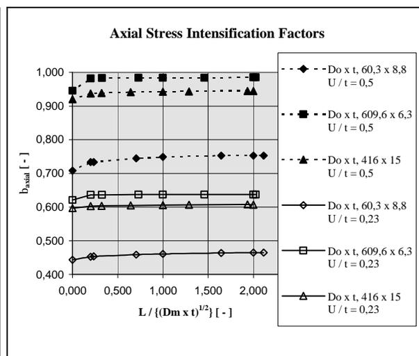
Figure 2: Axial SIFs, Internal Pressure,  $U/t=0,23$  and  $U/t=0,50$
