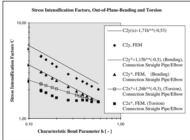
Figure 7: SIF, Connection Straight Pipe/Elbow, Out-of-Plane- Bending and Torsion
