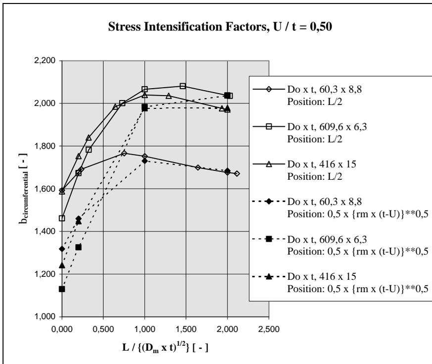
Figure 4: Circumferential SIFs, Internal Pressure,  $U/t=0,50$
