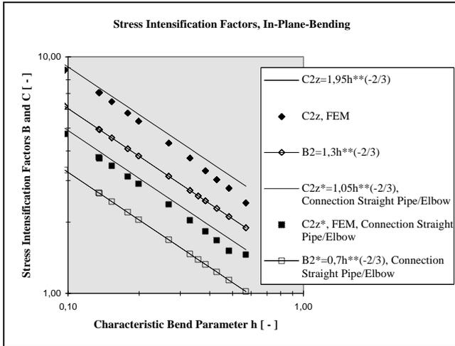
Figure 6: SIF, Connection Straight Pipe/Elbow, In-Plane-Bending
