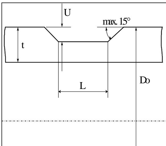
Figure 1: Circumferential undergrinding configuration
