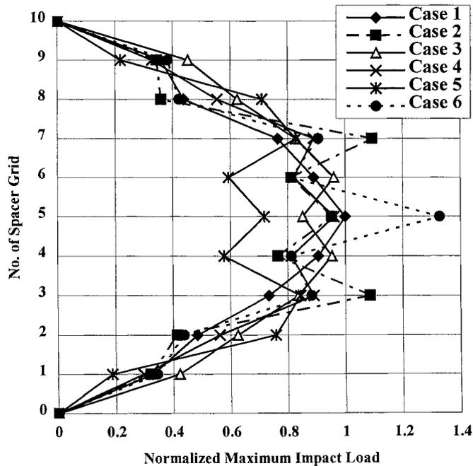
**Fig.4 Spacer Grid Impact Load Distribution along Fuel Assembly**
