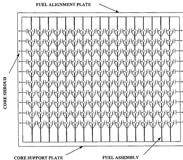
**Fig. 3 Typical Detailed Horizontal Core Model**
