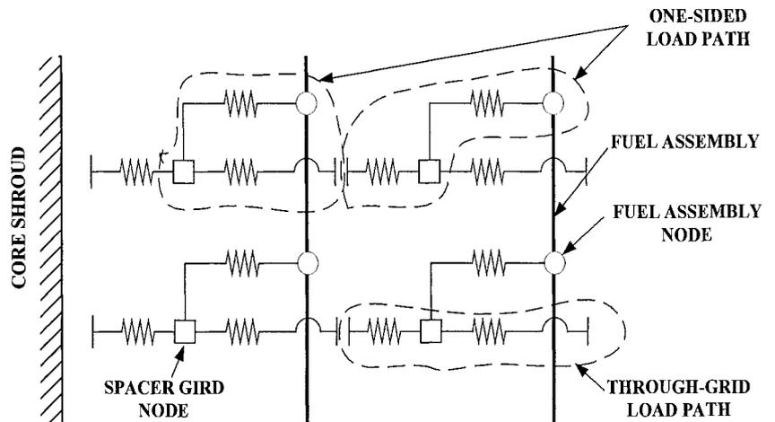
**Fig. 2 Typical Spacer Grid Spring Model**
