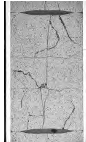
Fig. 2 Axial macrograph of a fuel rod irradiated for two annual PWR operating cycles
