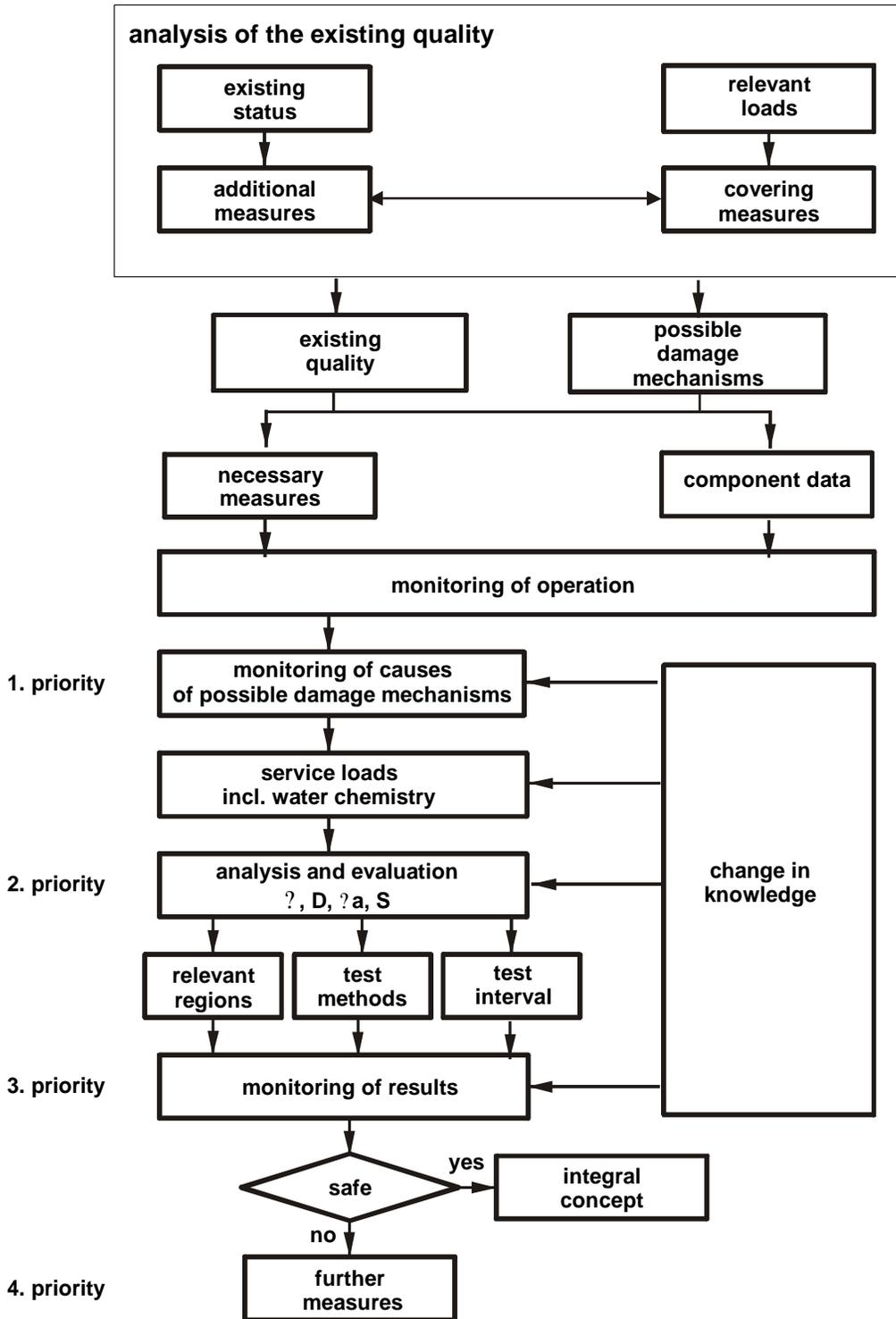
Fig. 5: Procedure to guarantee integrity of components
