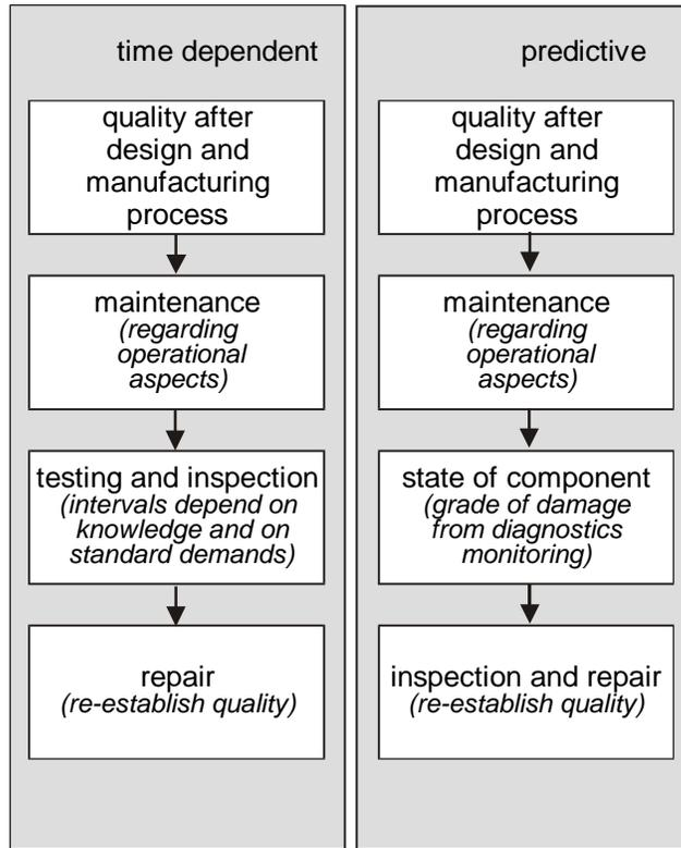
**Fig. 6: Procedure to maintain integrity and function**
