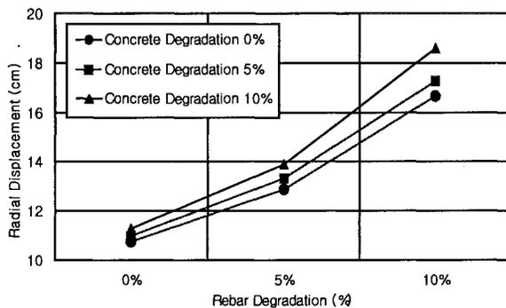
Fig. 8 Combination of concrete and rebar degradation
