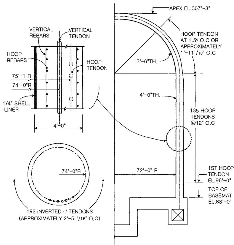
**Fig. 2 Axisymmetry Geometry of YGN #3 Containment**
