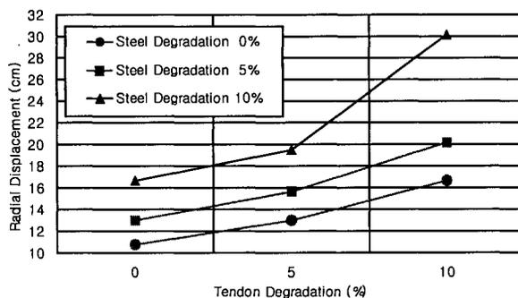
Fig. 10 Combination of rebar and tendon degradation
