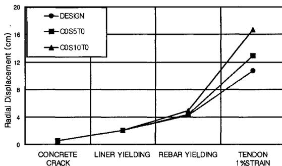
Fig. 6 Radial displacement by rebar degradation
