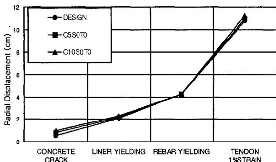
Fig. 5 Radial displacement by concrete degradation
