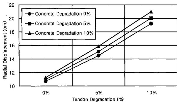
Fig. 9 Combination of concrete and tendon degradation
