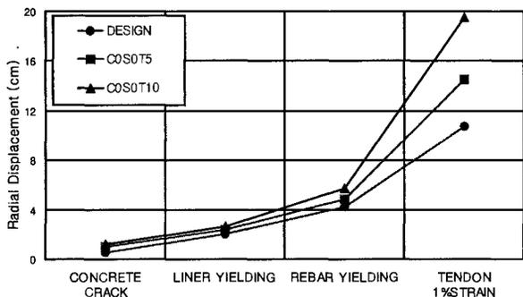
Fig. 7 Radial displacement by tendon degradation
