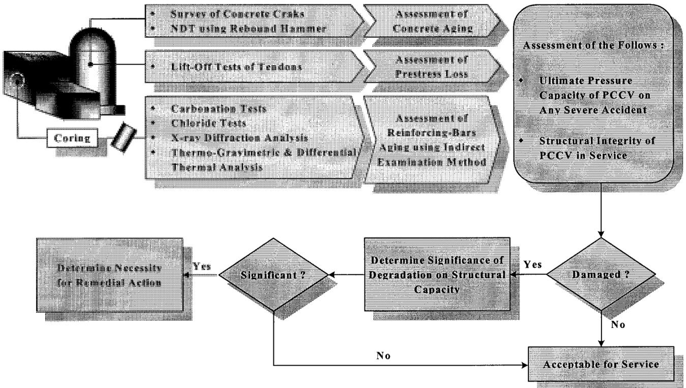
**Fig. 1. Structural integrity evaluation process for containment in service**
