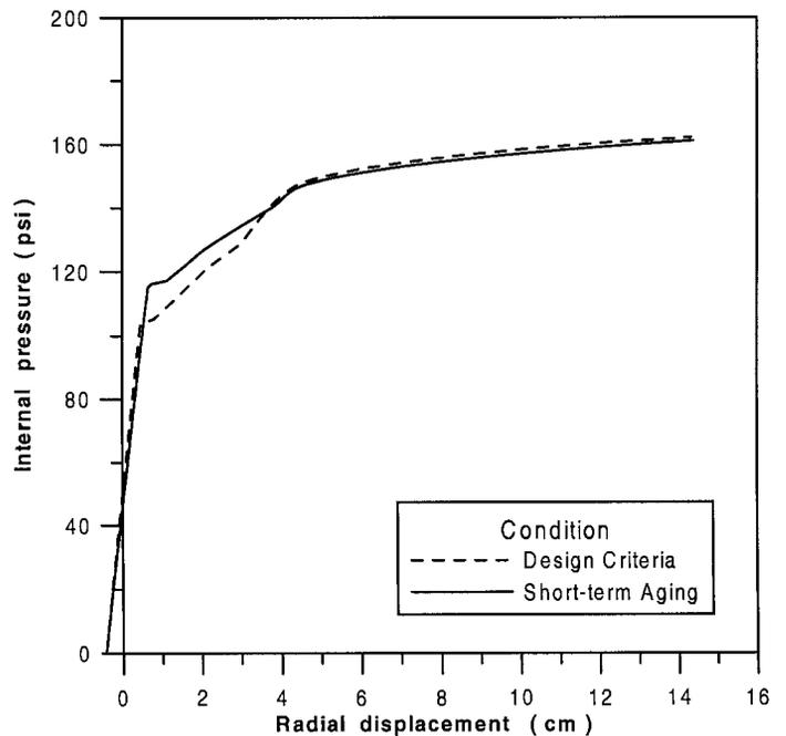
**Fig.4 Relationships between Internal Pressure and Radial Displacement at Mid-high Wall**
