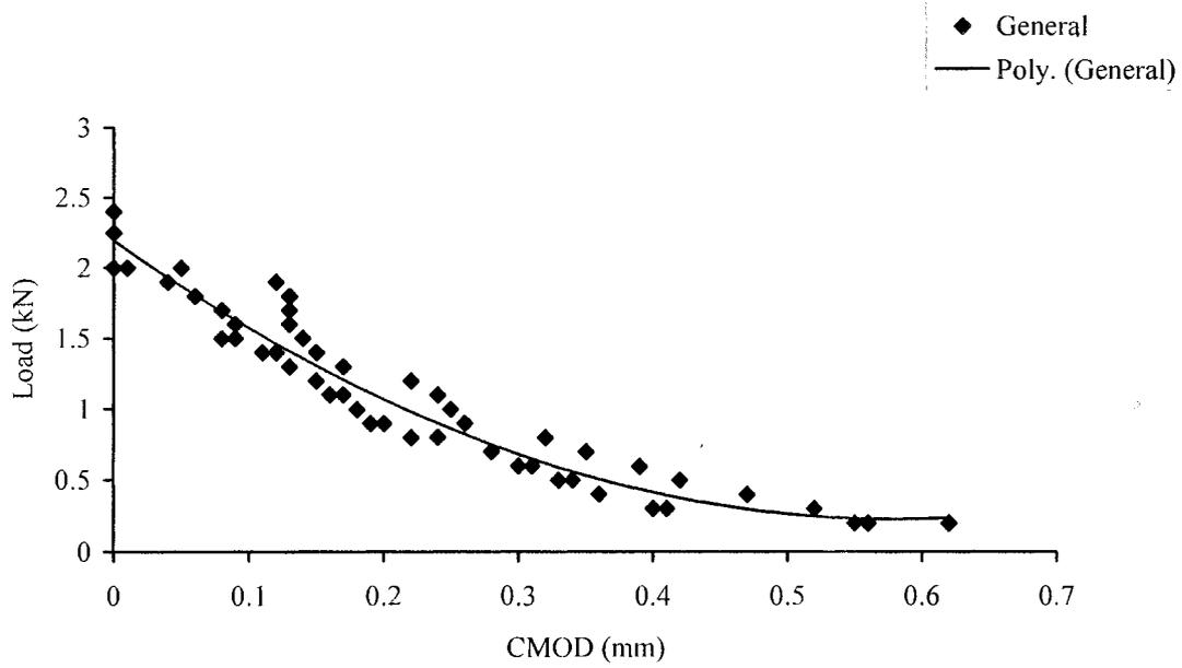
Fig. 9: General softening curve in HSC with  $w/b = 0.29$  .
