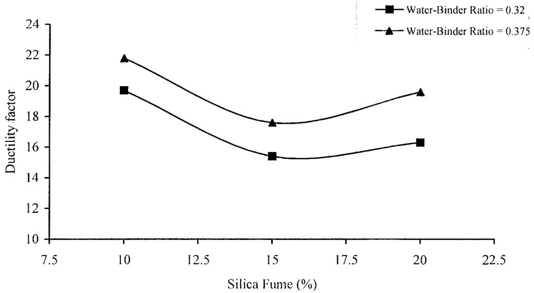
Fig. 8: Variation of ductility factor with silica fume content in HSC.
