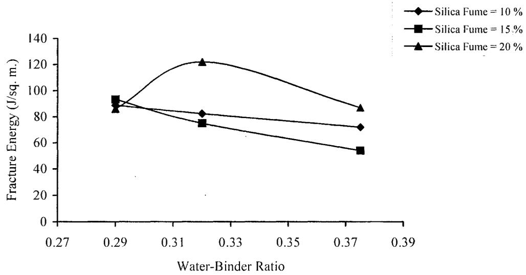
Fig. 3: Variation of fracture energy with water-binder ratio in HSC with different silica fume contents.
