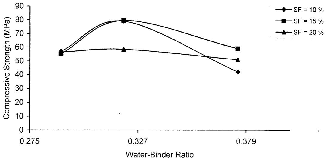
Fig. 1: Variation of compressive strength with water-binder ratio in HSC.
