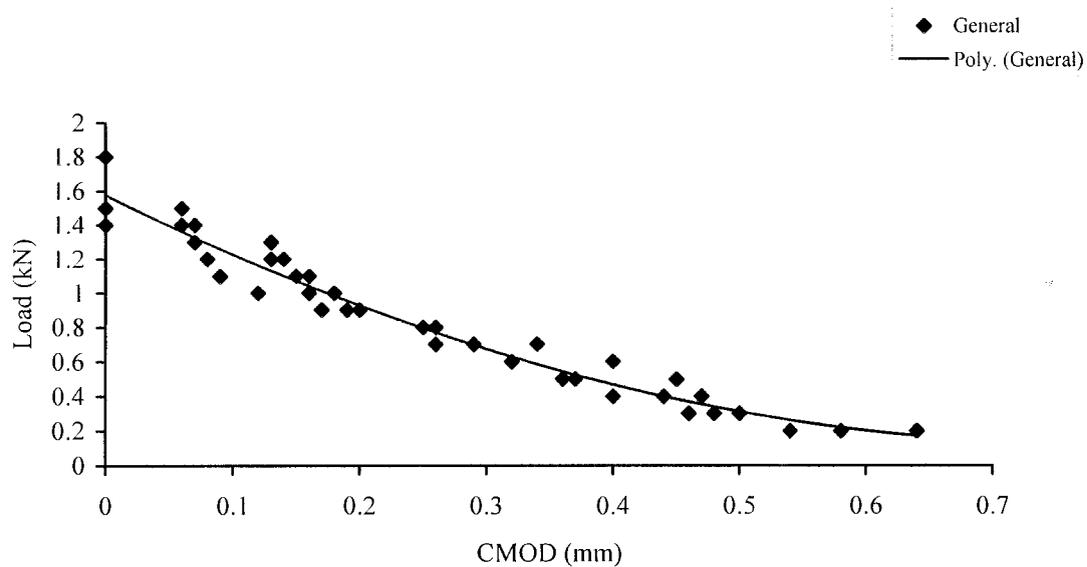
Fig.11: General curve for HSC with  $w/b = 0.375$ .
