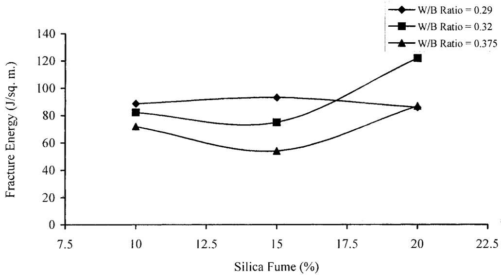
Fig. 4: Variation of fracture energy with silica fume content in HSC at different water-binder ratios.
