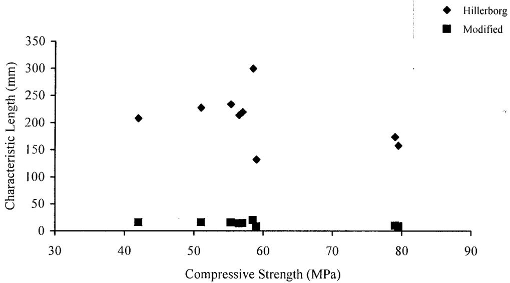
Fig.6: Variation of characteristic length with compressive strength in HSC.
