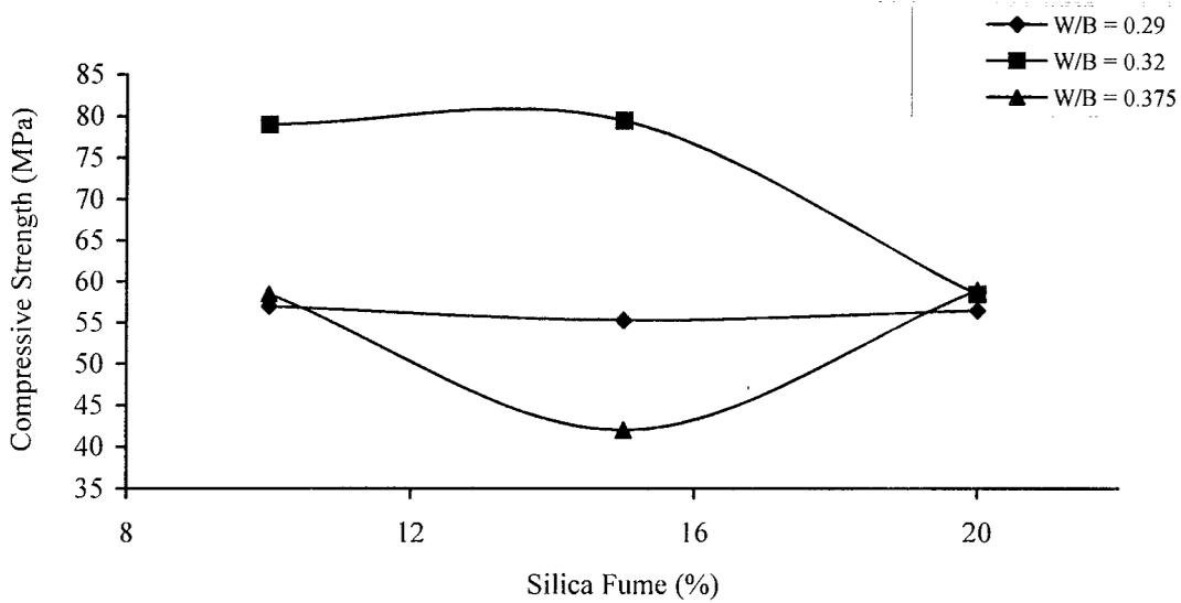
Fig. 2: Variation of compressive strength of HSC with silica fume at different w/b ratios.
