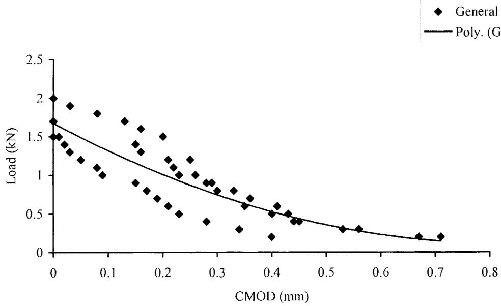
Fig. 10: General softening curve in HSC with  $w/b$  ratio = 0.32.
