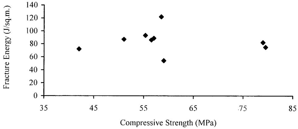
Fig.5: Variation of fracture energy with compressive strength of HSC with different silica fume contents at different w/b ratios.
