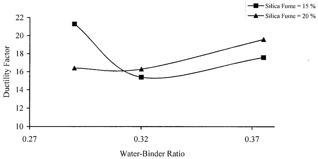
Fig. 7: Variation of ductility factor in HSC with water-binder ratio.
