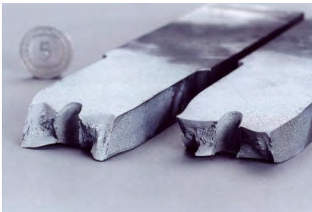
Fig. 5 Fracture surfaces of the 20 mm thick specimen
