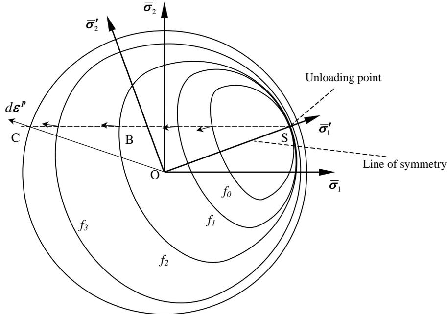
Fig. 2.2. Subsequent equi-plastic-strain surfaces and plastic strain increment directions
