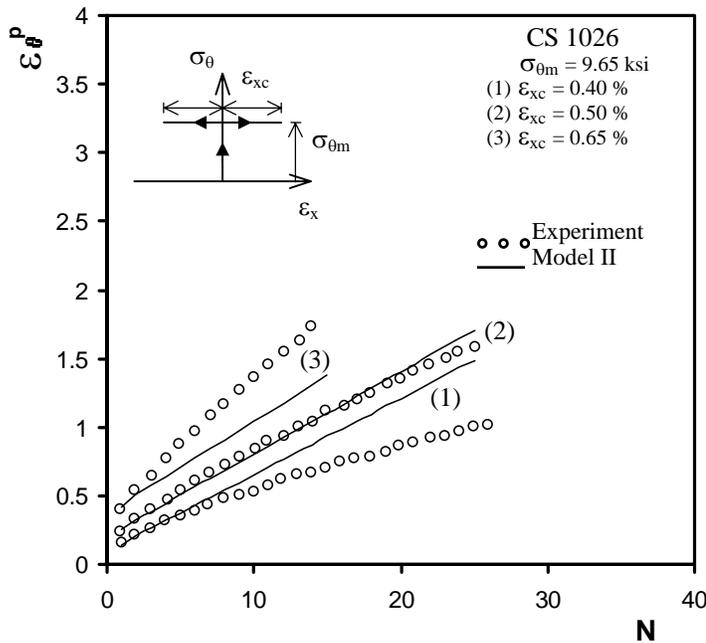
Fig. 2.6. Biaxial ratcheting predictions by model II and experiments from Hassan and Kyriakides [1992].
