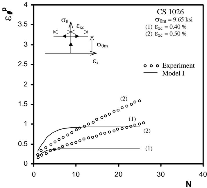
Fig. 2.4. Biaxial ratcheting predictions by model I and experiments from Hassan and Kyriakides [1992].
