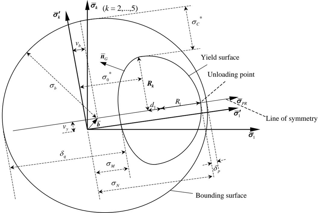
Fig. 2.3. Equi-plastic-strain surface I in the moving stress space  $\bar{\sigma}'_i$  of the Ilyushin space
