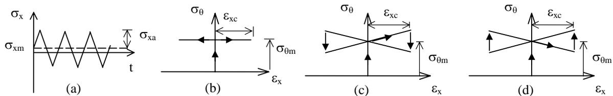
Fig 1.1 Loading histories; (a) Uniaxial stress cycles, (b) Axial strain cycle with constant pressure, (c) biaxial bow-tie cycle, (d) biaxial reverse bow-tie cycle.
