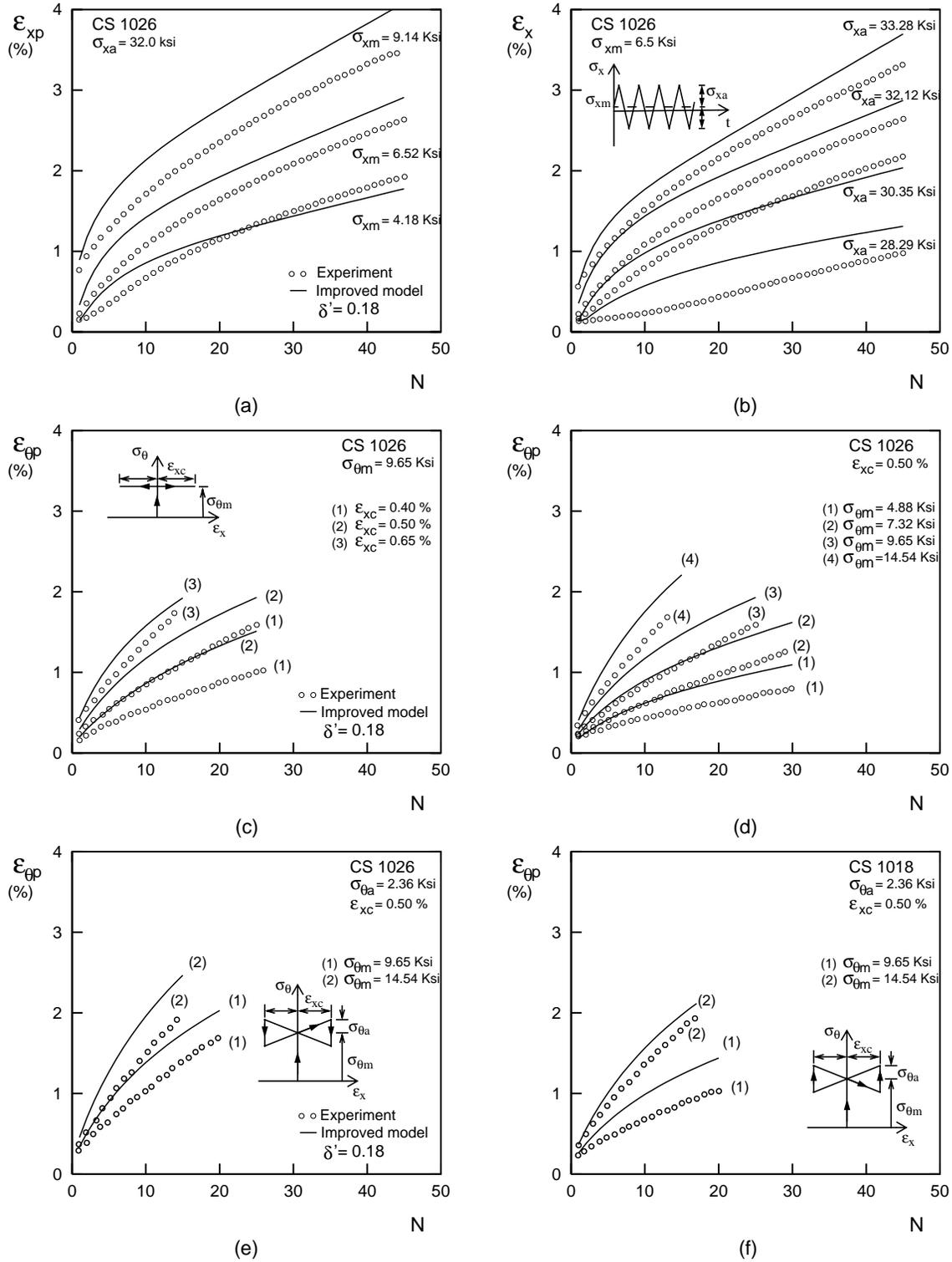
Fig. 1.2. Ratcheting predictions by the Improved model (Eq. 16). (a,b) Axial strain at positive stress peaks from uniaxial cycles, (c,d) circumferential strain peaks from axial strain cycles with constant pressure, (e,f) circumferential strain peaks from bow-tie and reverse bow-tie cycles. Experiments are from Hassan and Kyriakides (1992), Hassan et al. (1992) and Corona et al. (1996).
