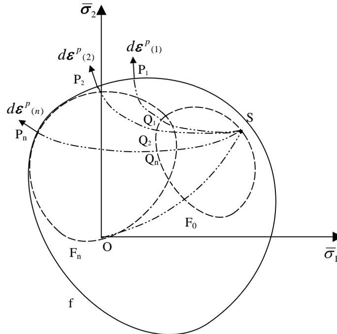
Fig. 2.1 Qualitative equi-plastic-strain surface in Ilyushin [1954] vector stress space
