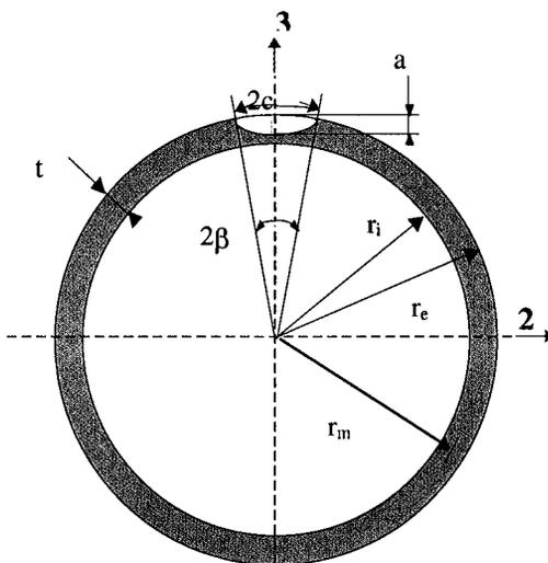
Figure 1 - A semi-elliptical circumferential crack in a pipe
