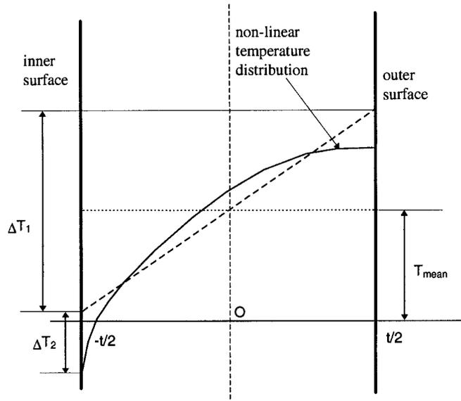
Figure 7 - Through wall temperature distribution in a pipe
