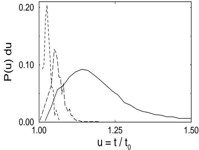
Figure 5: Distribution of the ratio of lifetime,  $t$ , when interaction are taking into account to the lifetime,  $t_0$ , in the absence of interactions. The data were obtained using 600 initial crack configurations generated using self-affine profiles made of facets of different slopes  $s$ . Solid, dotted and long dashed lines correspond respectively to  $s = 0.1$ ,  $0.01$  and  $0.001$ . The crack velocity law used is  $v(K_I) = \exp(K_I)$  and  $K_{Ic} = 1$ .
