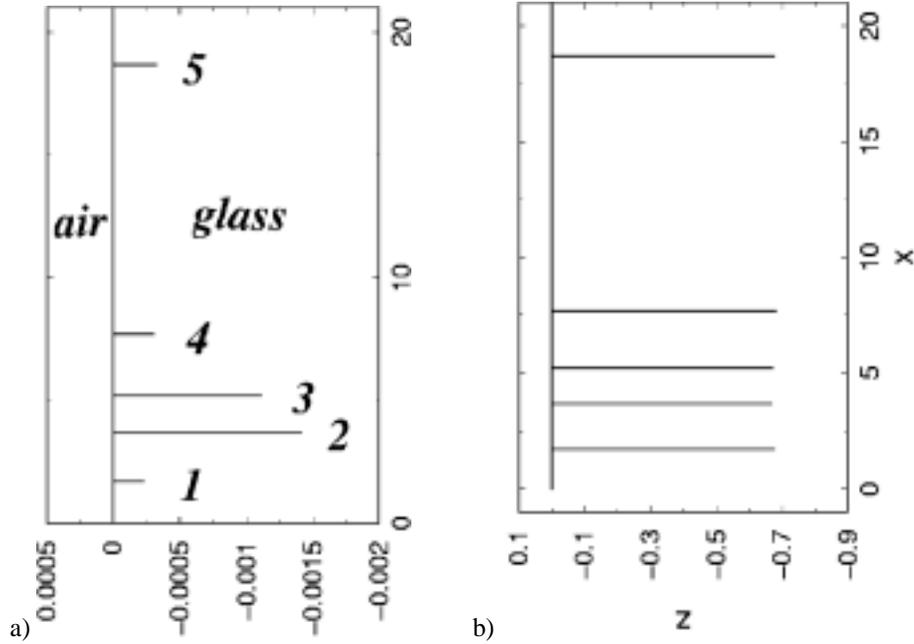
Figure 3: The figure (a) shows the initial crack configuration, consisting of  $N = 5$  cracks load by a remote tension  $\sigma_0 = 1$ . Figure (b) represents the cracks when  $K_{Ic}$  is reached. In this simulation the speed of the crack is  $v(K_I) = \exp(K_I)$  and  $K_{Ic} = 1$ . Initially the ratio between the average crack length and the distance separating them is  $\langle a \rangle / b = 4.10^{-3}$  and is  $\langle a \rangle / b = 0.28$  when failure occurs.
