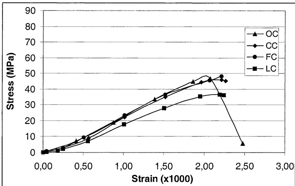
Fig. 5 Stress-strain relationships of the tested concretes after exposure at 200 °C and cooled down.
