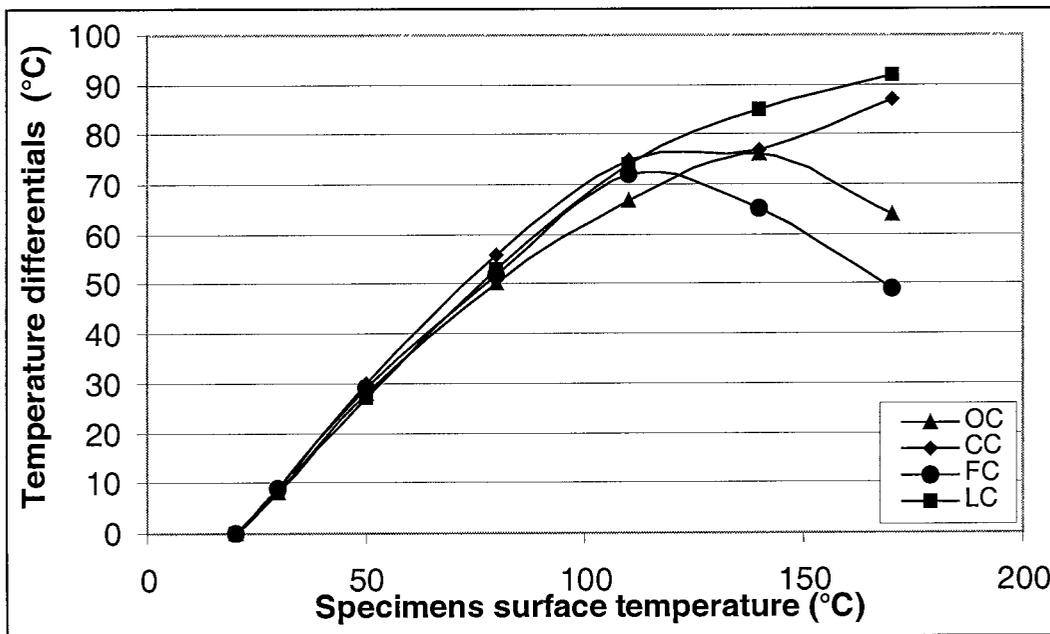
Fig. 3 Temperature differentials between the surface and the centre of the 16x32 cm concrete specimens
