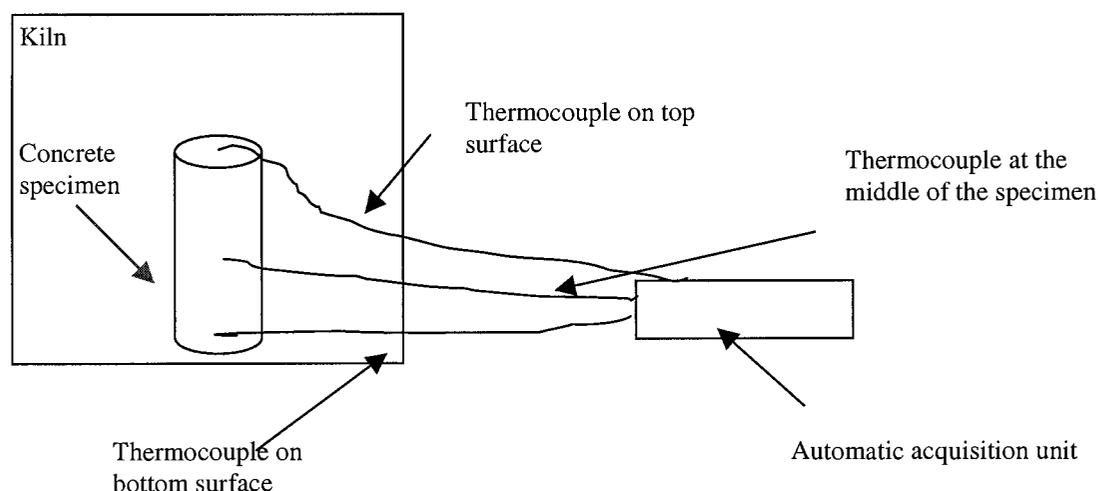
Fig. 1 Location of surface temperature measuring points
