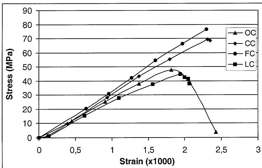
Fig. 4 Stress-strain relationships of the tested concretes at room temperature
