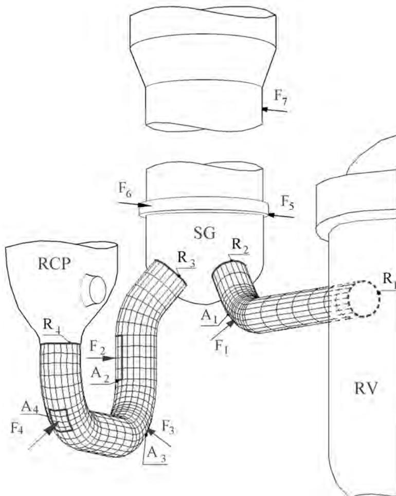
**Fig. 1 Hot and crossover leg of the primary piping modelled with shell elements**
