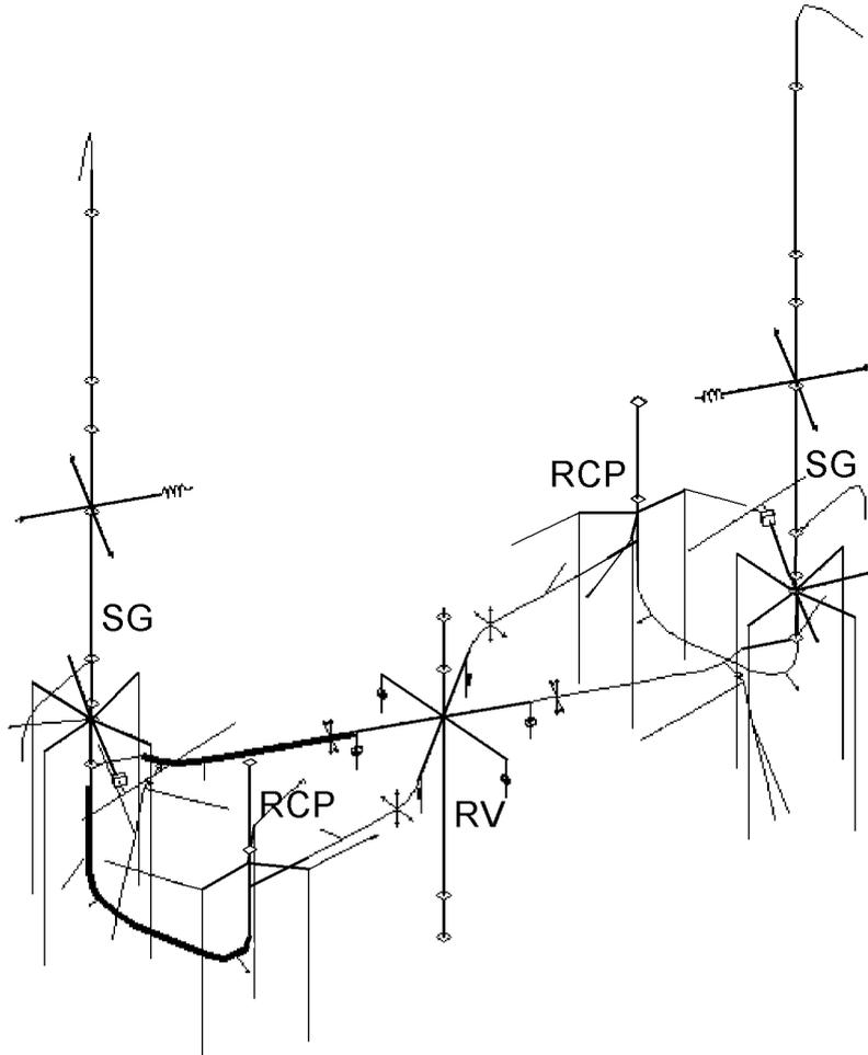
**Fig. 2 Two-loop reactor coolant system modelled with beam elements**
