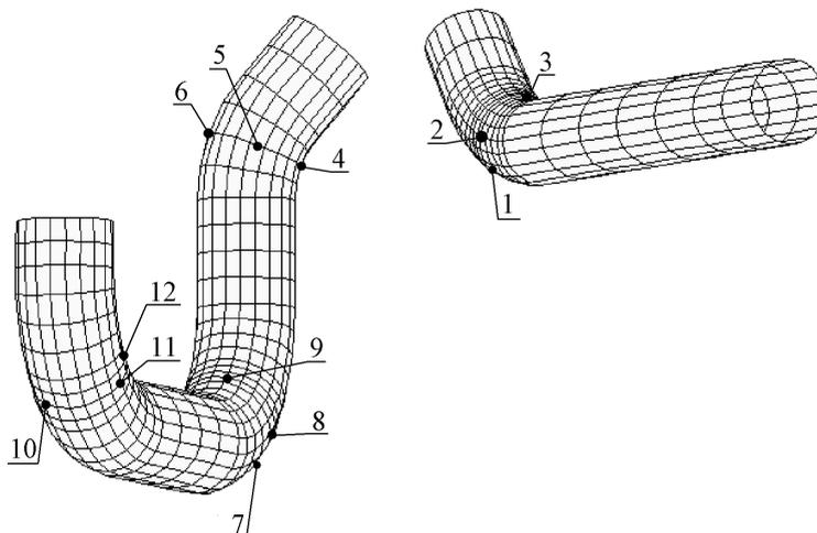
**Fig. 3 Position of critical points on hot and crossover leg**
