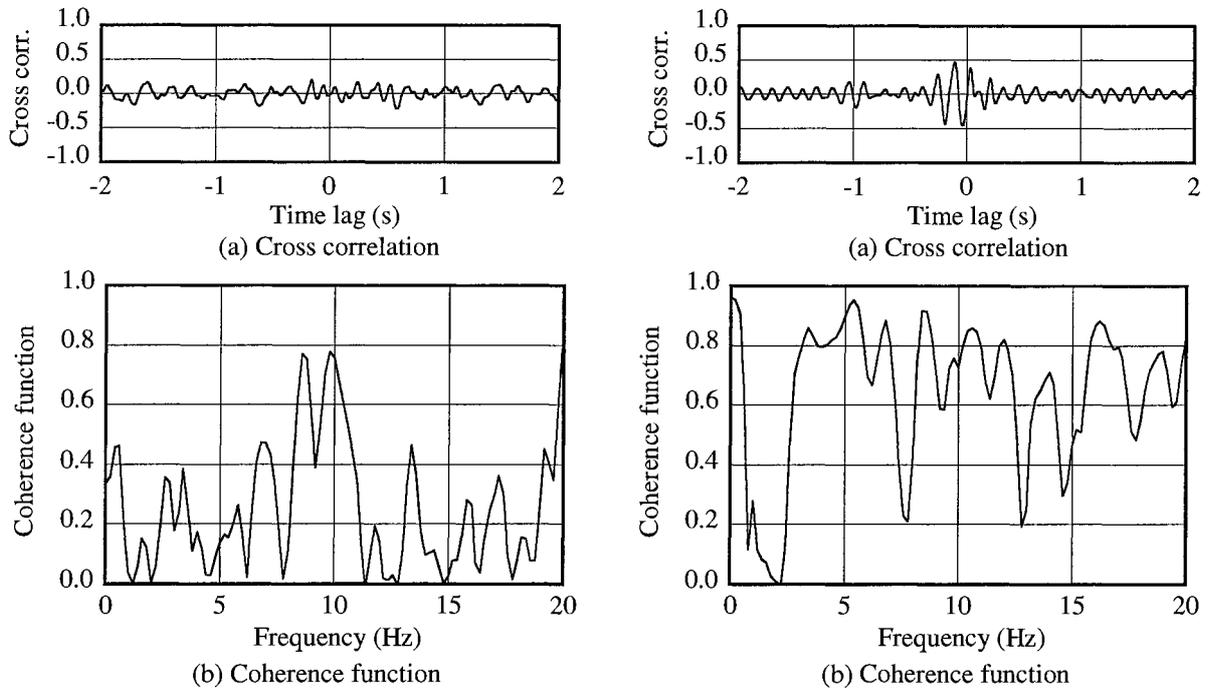
Fig.3 Examples of cross correlation and coherence function. Left figure shows low coherency (Event 14), and right is high coherency (Event 7).
