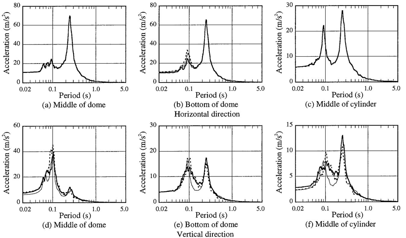
Fig.9 5% damped acceleration response spectra (vertical input motion have inverse phase to the case of Figure 8)
