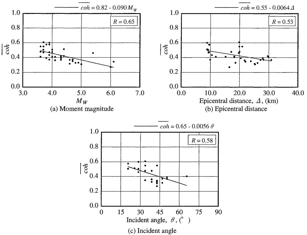
Fig.4 Relationships between seismic parameters and average coherence
