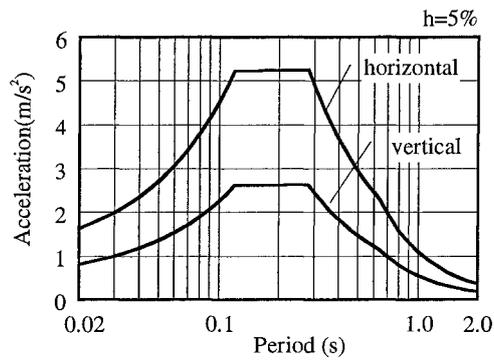
Fig.6 Target spectra of artificial input waves
