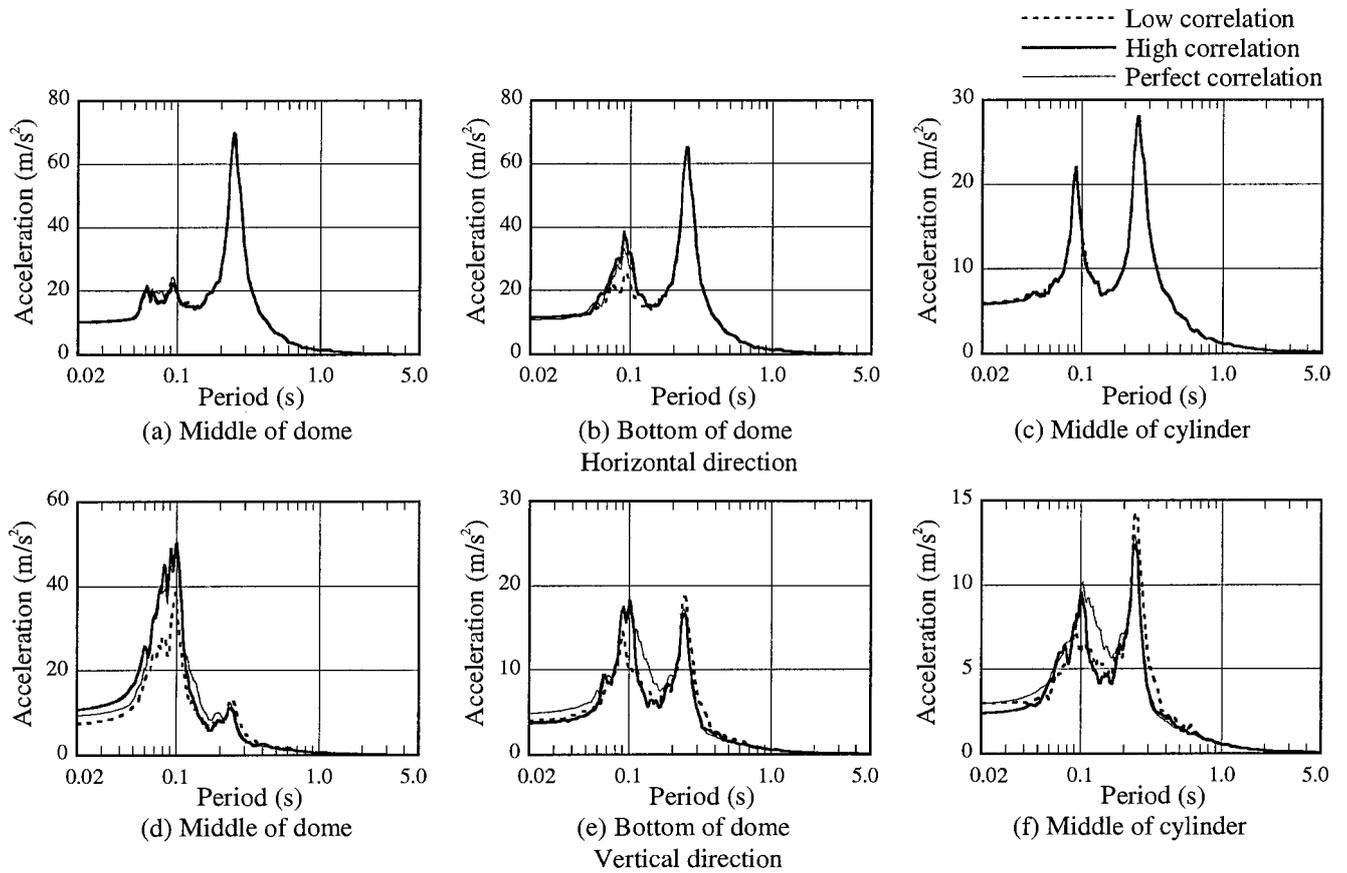
Fig.8 5% damped acceleration response spectra due to correlated horizontal and vertical input motions
