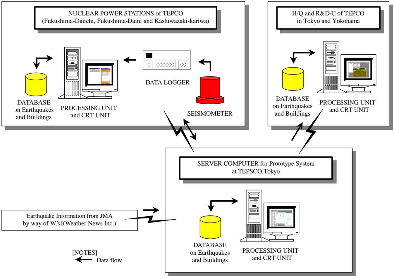
**Fig.1 The Outline Composition of Prototype System**
