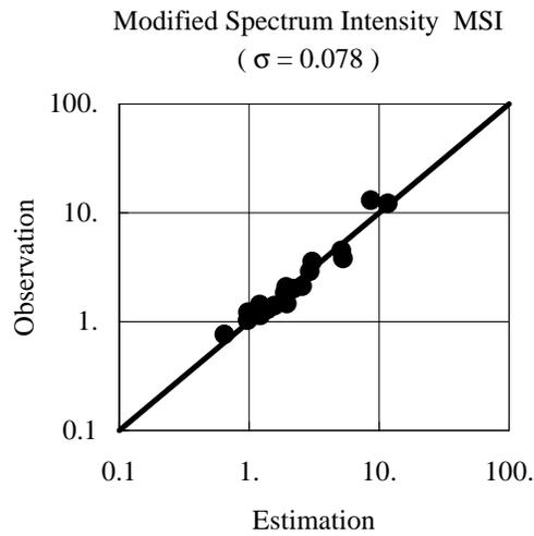
**Fig.4 The Comparison Between Observation and Estimation in Indexes of Earthquake Motion Intensity**
