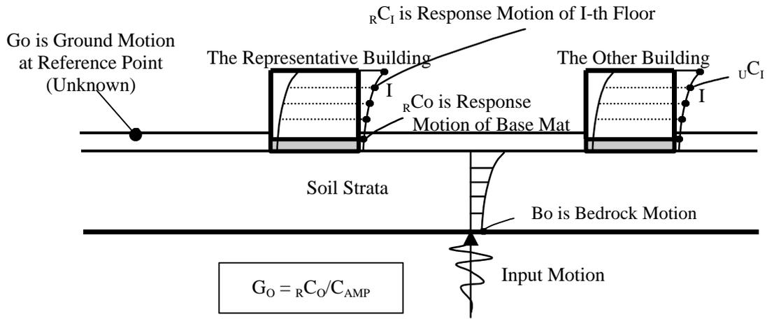
**Fig.2 (b) Response Motions Calculated by Dynamical Response Analysis**
