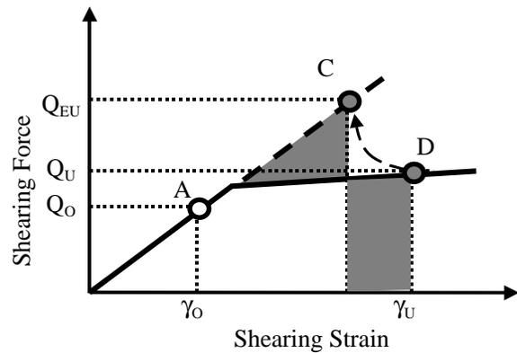
**Fig.3 (b) The Equivalent Ultimate Strength  $Q_{EU}$  based on the Energy Equivalence Assumption**
