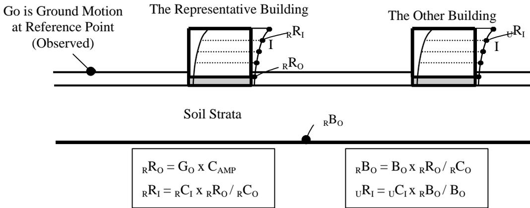
**Fig.2 (c) Response Estimation based on the Observation Record of Reference Point**
