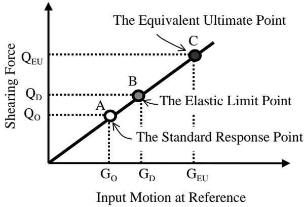
**Fig.3 (c) The Enhanced Damage Estimating Function with Points B and C**
