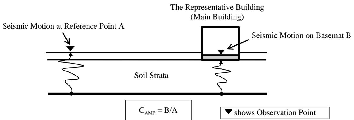
**Fig.2 (a) The Building Amplification Coefficient  $C_{AMP}$  based on The Earthquake Observation Records**
