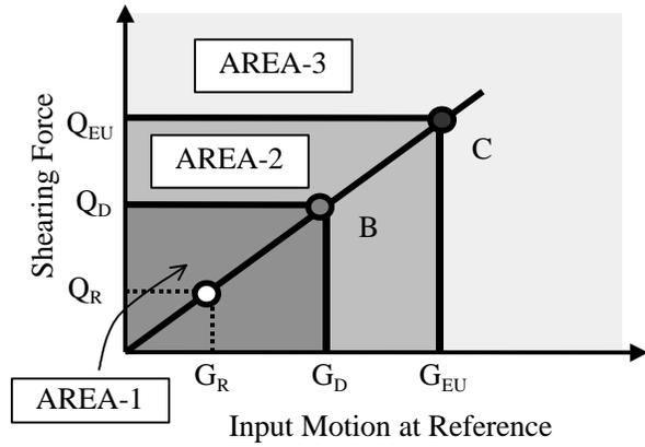
**Fig.3 (d) The Three Rank Damage Area Classified According to the Damage Estimating Function**
