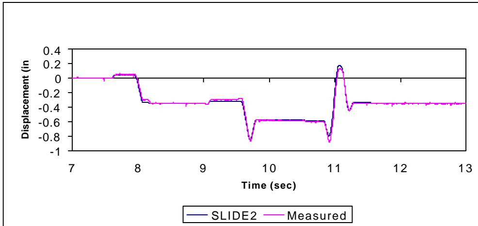
**Figure 8. Best simulation from SLIDE2: 1971 San Fernando earthquake with reversed polarity.**
