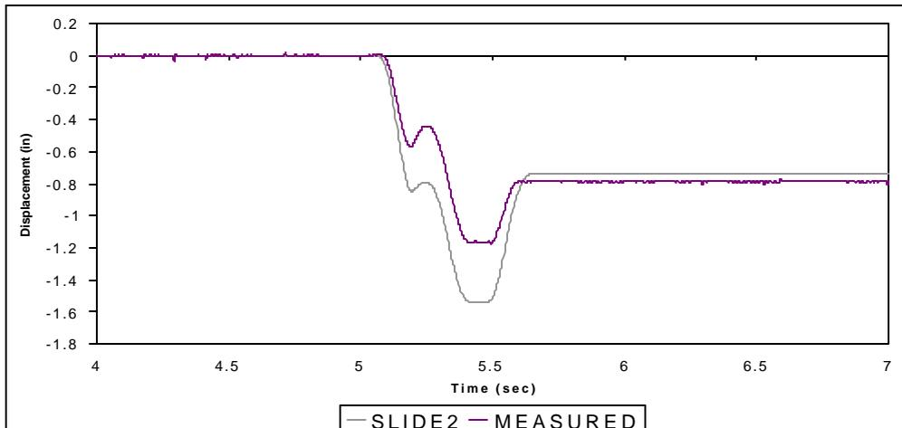
**Figure 9. Best simulation from SLIDE2: 1966 Parkfield earthquake**
