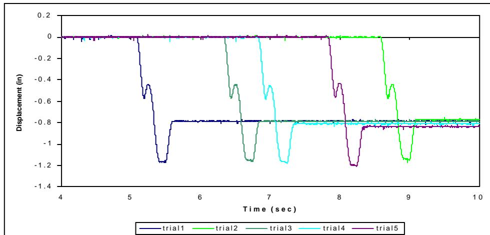
Figure 4. Repeatability results with final experimental setup: 1966 Parkfield Excitation
