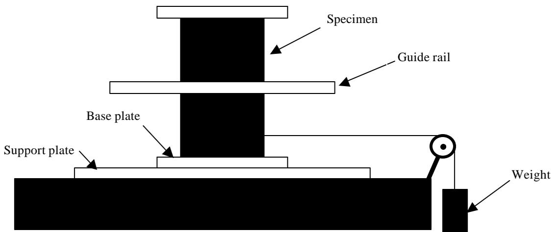
Figure 1. Sketch of the quasi-static pulley test to determine the coefficients of friction
