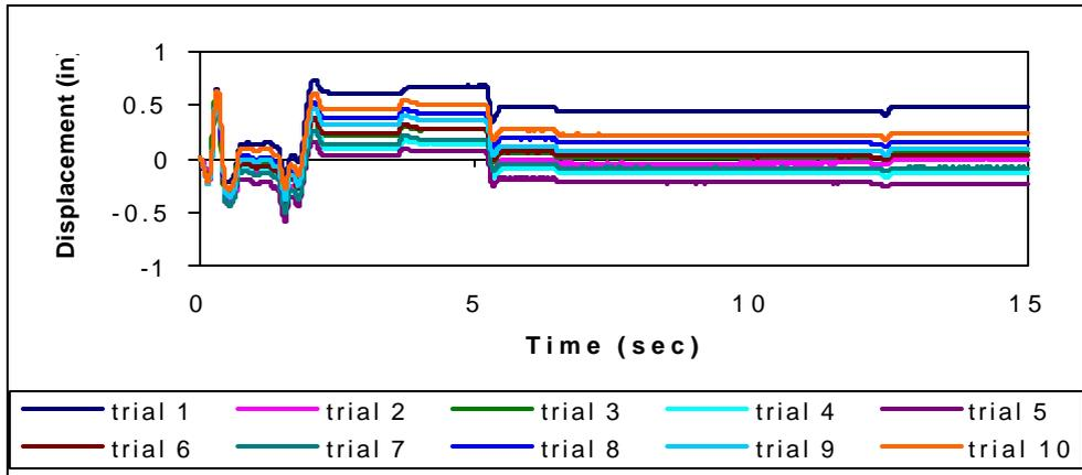
Figure 3 Repeatability results with initial experimental setup: 1940 Imperial Valley Excitation
