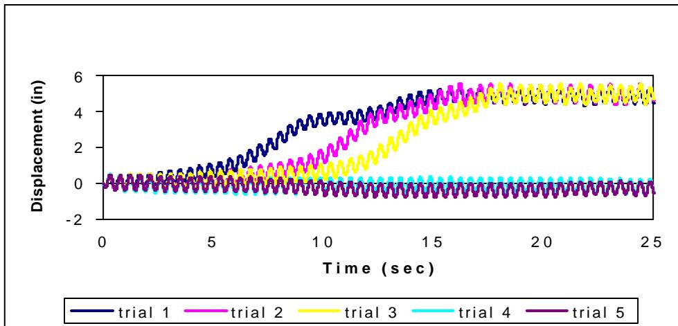
**Figure 2 Repeatability results with initial experimental setup: 2 Hz Sinusoidal Excitation**
