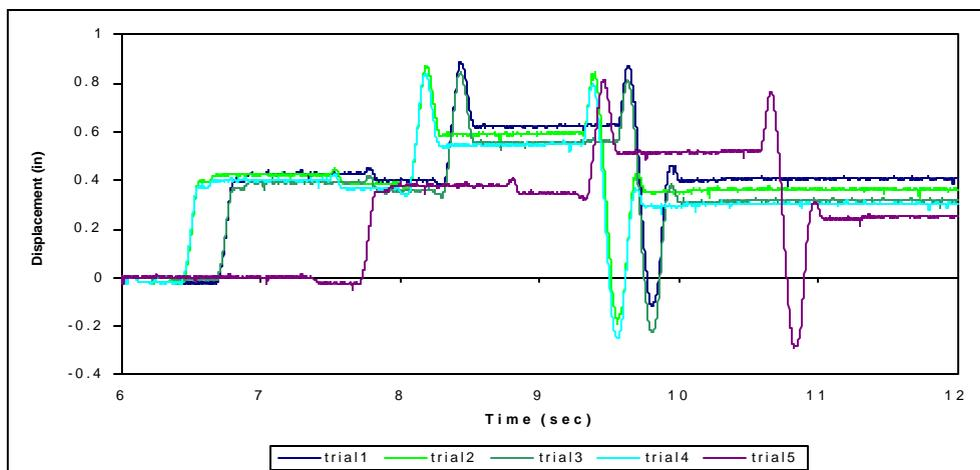
Figure 5. Repeatability results with final experimental setup: 1971 San Fernando Excitation
