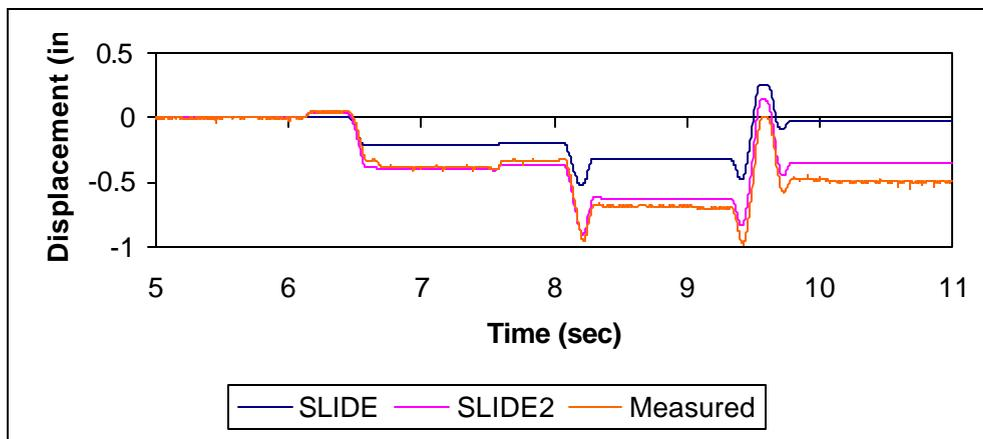
Figure 6. Measured and calculated responses from SLIDE and SLIDE2: 1971 San Fernando Excitation.
