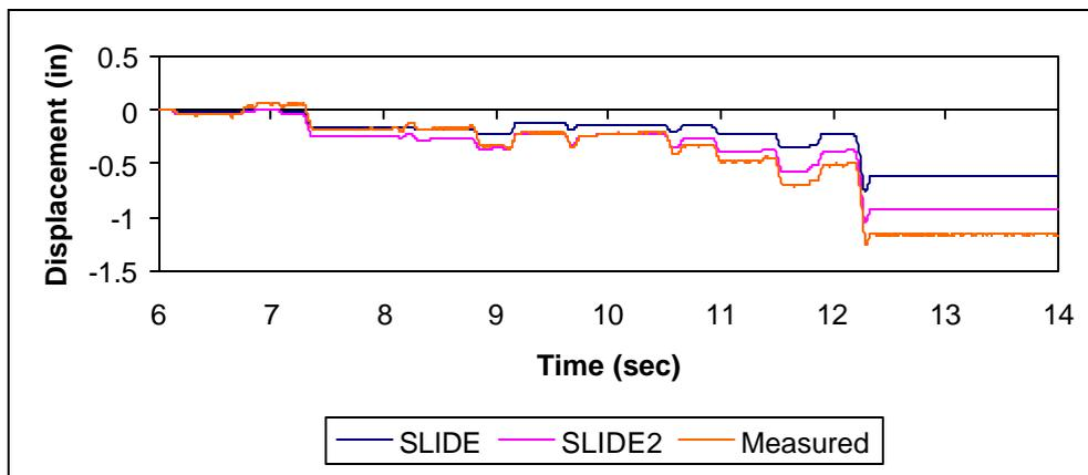
Figure 7. Measured and calculated responses from SLIDE and SLIDE2: 1949 Western Washington Excitation.
