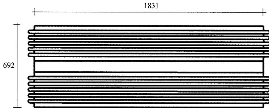
Figure 2 Vent line bellows (dimensions in mm)
