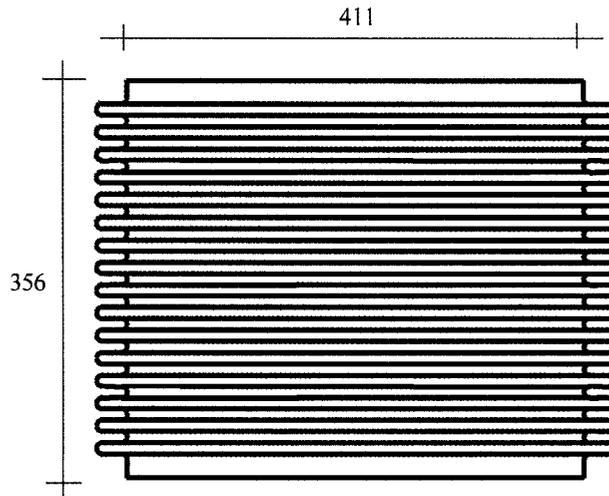
Figure 3 Vacuum breaker bellows (dimensions in mm)
