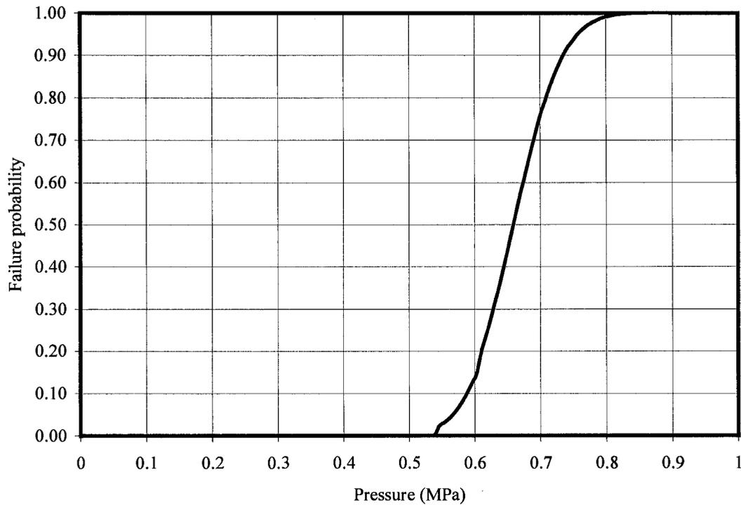
Figure 6 Fragility curve of the containment
