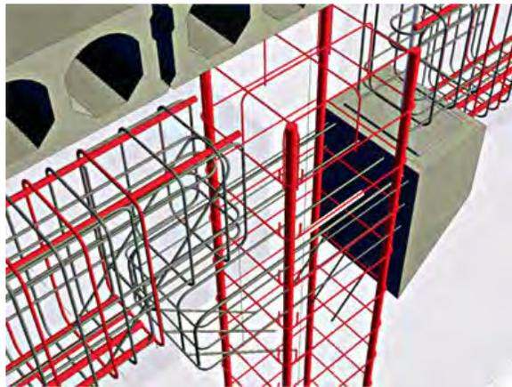
Figure 4 Typical Detail of a Cast-in-place Concrete Model
