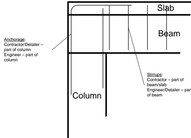
**Figure 3 Column-beam-slab Connection**
