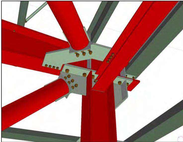
**Figure 2 Typical Detail of a Structural Steel Model**
