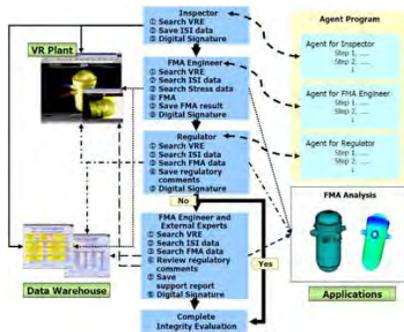
Fig. 5 Integrity assessment procedure using the agent program
