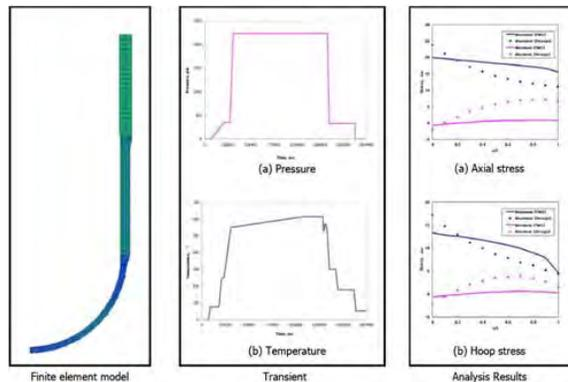
Fig. 4 An example of structural analysis on RPV
