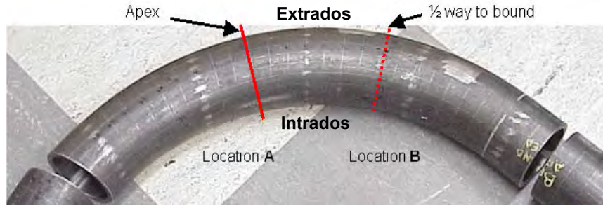
Figure 3 Bent Feeder Pipe [3]
