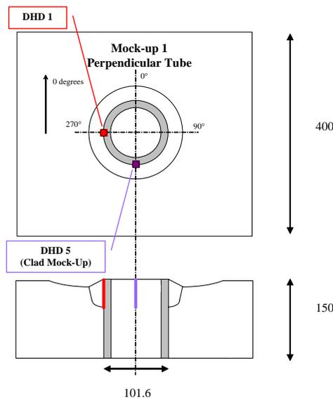
**Figure 2. Mock-up 1: central nozzle general arrangement, DHD locations and dimensions (mm)**
