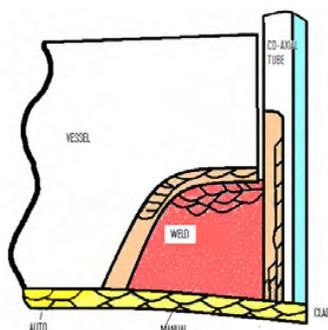
Figure 1. Schematic of J-groove weld
