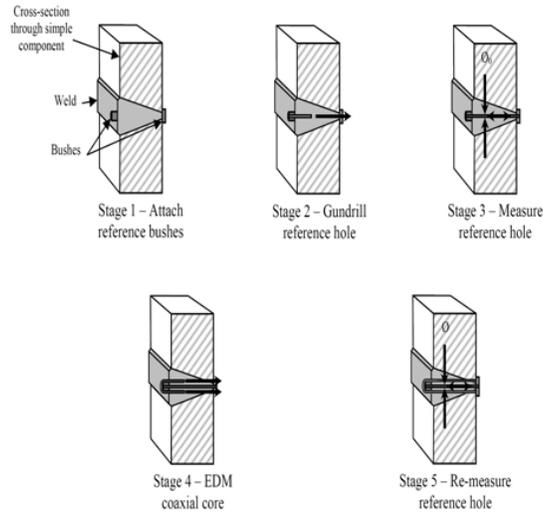
**Figure 5. Stages in the deep hole drilling residual stress measurement method**
