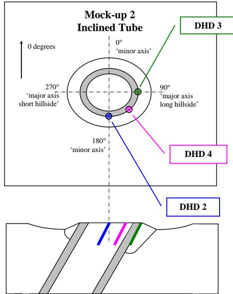
Figure 3. Mock-up 2: off-centre nozzle general arrangement and DHD locations
