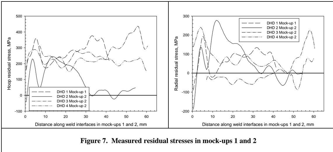
**Figure 7. Measured residual stresses in mock-ups 1 and 2**
