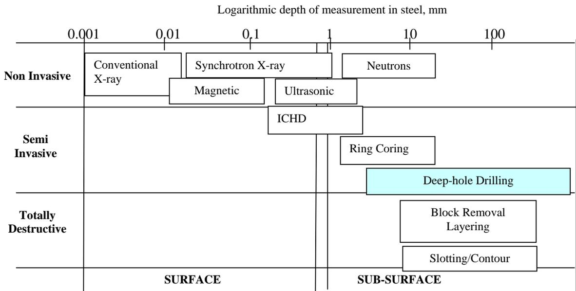
Figure 4. Residual stress measurement methods in steel.
