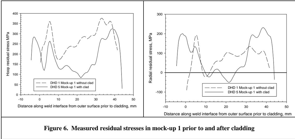
**Figure 6. Measured residual stresses in mock-up 1 prior to and after cladding**
