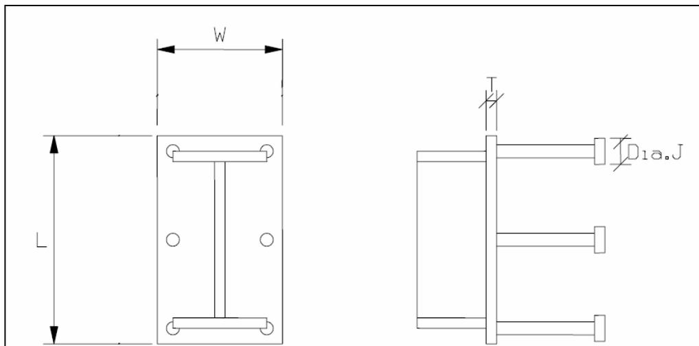
**FIGURE 4.** Example of a Typical AP1000 Embedment Plate.
