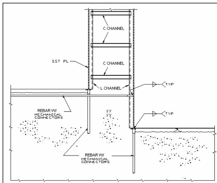
**FIGURE 2.** Typical Base Detail for AP1000 Wall Modules
