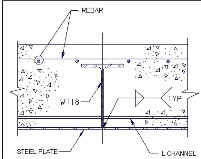
**FIGURE 3.** Typical AP1000 Floor Structural Module
