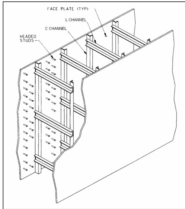
**FIGURE 1.** Typical AP1000 Structural Wall Module Detail
