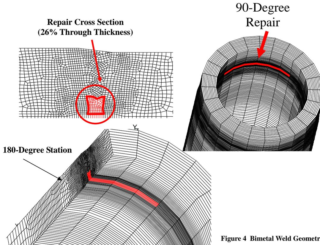
Figure 4 Bimetal Weld Geometry.
