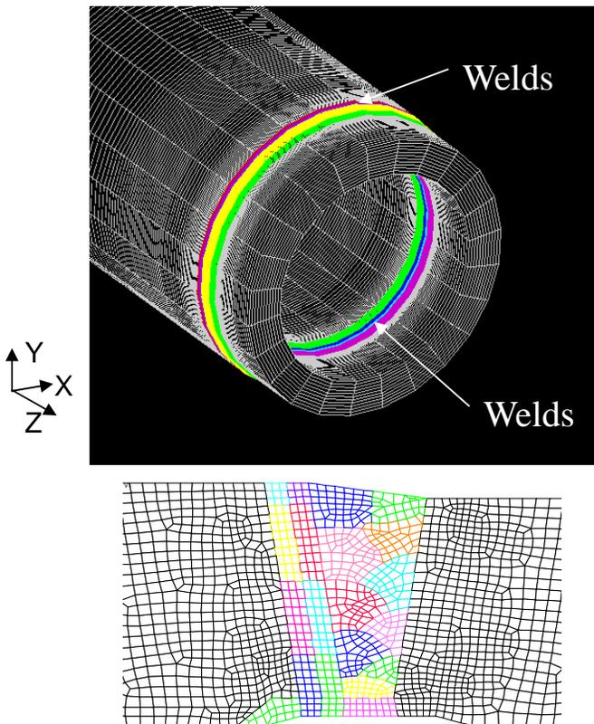
Figure 3 Bimetal Weld Geometry.
