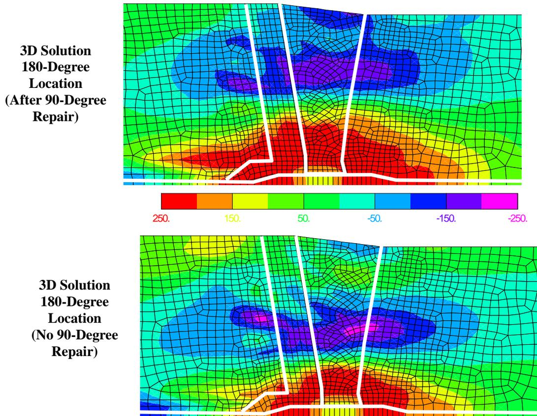
**Figure 5. Axial Stresses – Welding 90-Degree Repair T = 324C**
