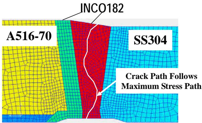
Figure 1 Crack path following maximum stress in
