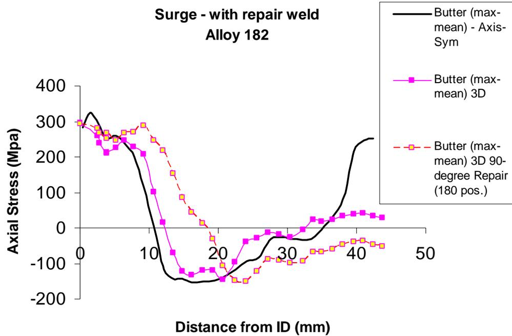
Figure 6. Axial Stresses – Welding Original 360 Grind and Repair (T = 324C)
