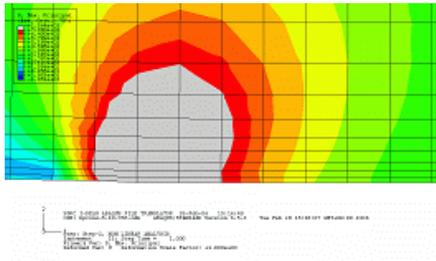
Fig. 9 Plastic zone in the case of a hydride of 10 μm (Stage II,  $K=7.88MP\sqrt{m}$ )
