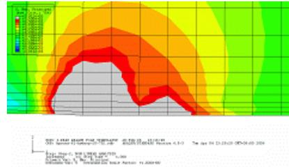
Fig. 11 Plastic zone in the case of a hydride growth of 20 μm (Stage I,  $K=7.52MP\sqrt{m}$ )
