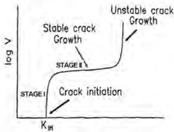
Figure 1. Dependency of the crack growth velocity with K.
