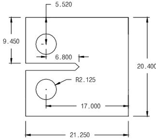
Figure 5. The Dimensions of the CT specimen.
