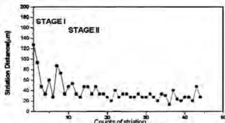
Figure 3. Variation of the striation spacing of a DHC.
