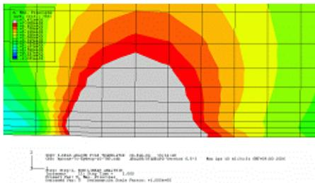
Fig. 12 Plastic zone in the case of hydride 10 μm when considering a hydride expansion (Stage II,  $K=7.88MP\sqrt{m}$ )
