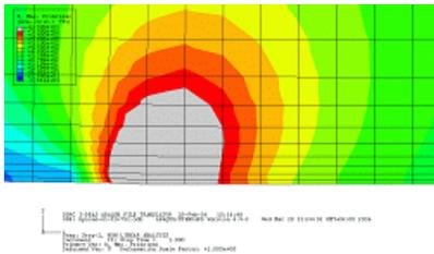
Fig. 7 Plastic zone in the case of a hydride growth of 10 μm (Stage I, K=7.52MP√m)
