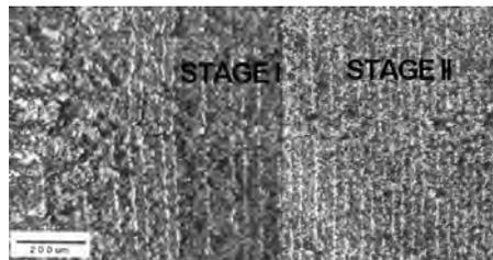
Figure 2. Striation lines on the fractured surfaces of the DHC CT specimen
