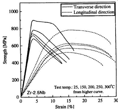
Figure 4. Tensile stress-strain curves in the transverse and longitudinal directions of the specimens
