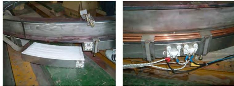
(a) Heating Plate (b) Setup for Heating Plates and Cooling Coils
