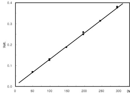
Figure 4. Voltage from the Strain Gauge depending on Thermal Loads
