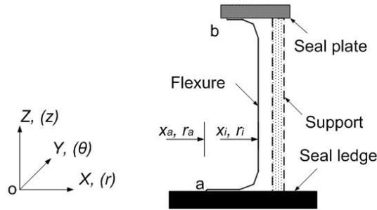
Figure 1. Section of a Test Model
