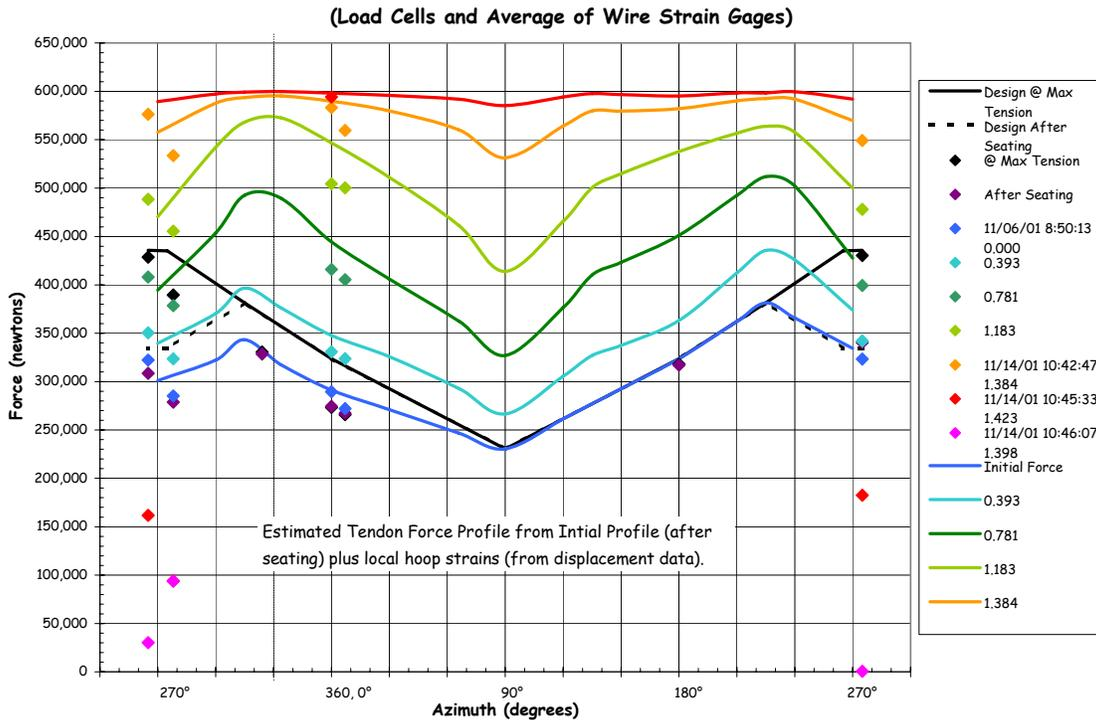
Figure 3 SFMT – Tendon H35 Computed and Measured Force Distribution
