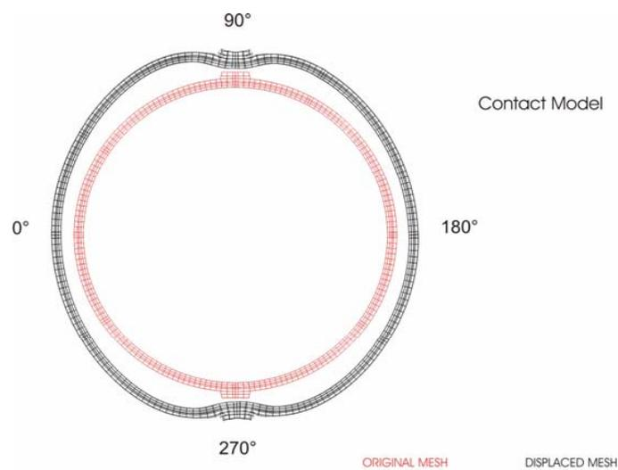
**Figure 6** Comparison of Deformed Shapes (displ. x 200) Using Tendon Friction Truss Ties vs. the Contact Surface Model at  $P=2.0P_d$
