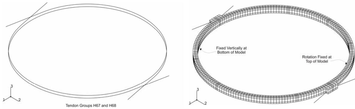
**Figure 4 Ring Model Tendons and Boundary Conditions**
