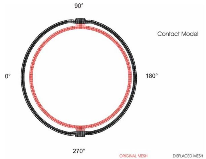
**Figure 7** Comparison of Deformed Shapes (displ. x 20) Using Tendon Friction Truss Ties vs. the contact Surface Model at  $P=3.5P$
