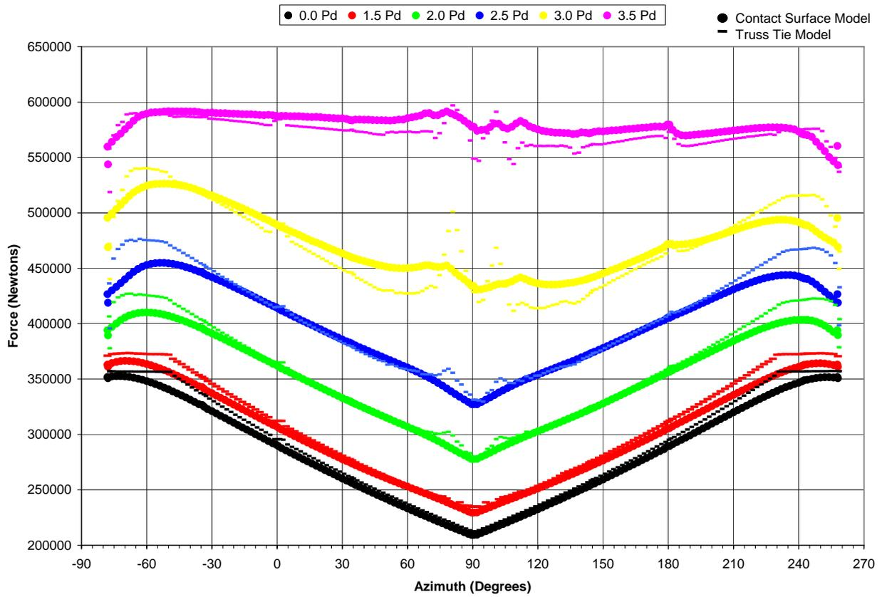
**Figure 5 Comparison of Tendon Force Distributions for Two Tendon Friction Modeling Strategies**
