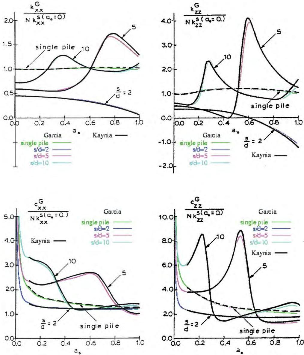
**Figure 3. Dynamic stiffnesses of single pile and pile group under externally applied harmonic forces. Top left: horizontal excitation, real component; top right: vertical excitation, real component; bottom left: horizontal excitation, imaginary component; bottom right: vertical excitation, imaginary component.**
