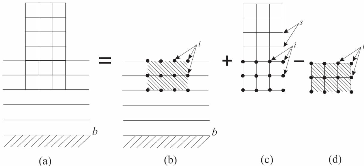
**Figure 1. Substructures of the system: (a) total system; (b) soil deposit; (c) structure; (d) excavated soil (modified after Lysmer et al., 1988)**
