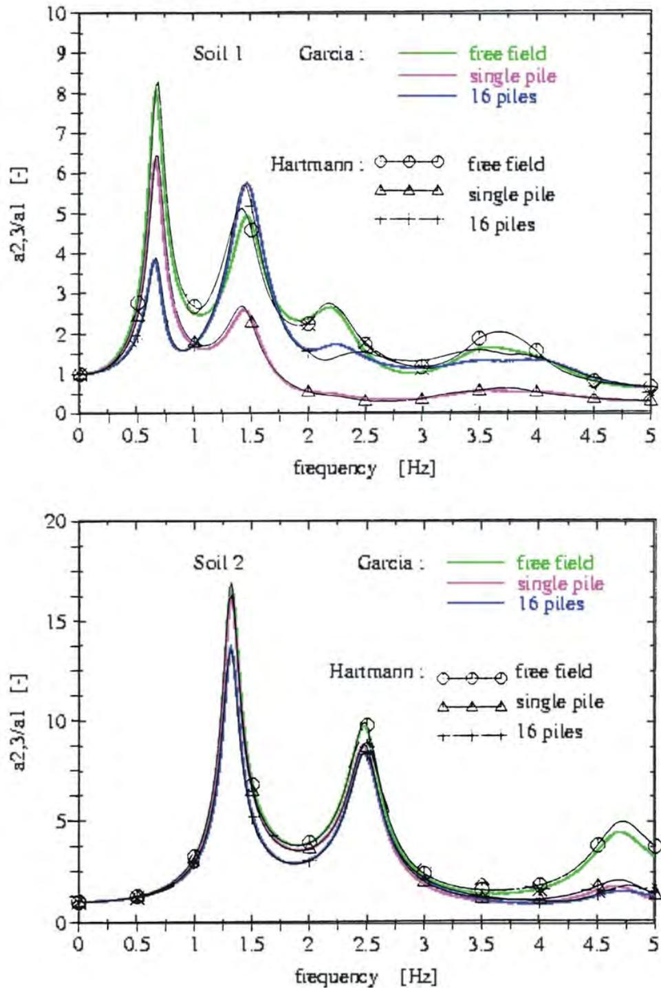
**Figure 4. Horizontal harmonic foundation top response functions under harmonic seismic excitation: top: soil 1; bottom: soil 2.**
