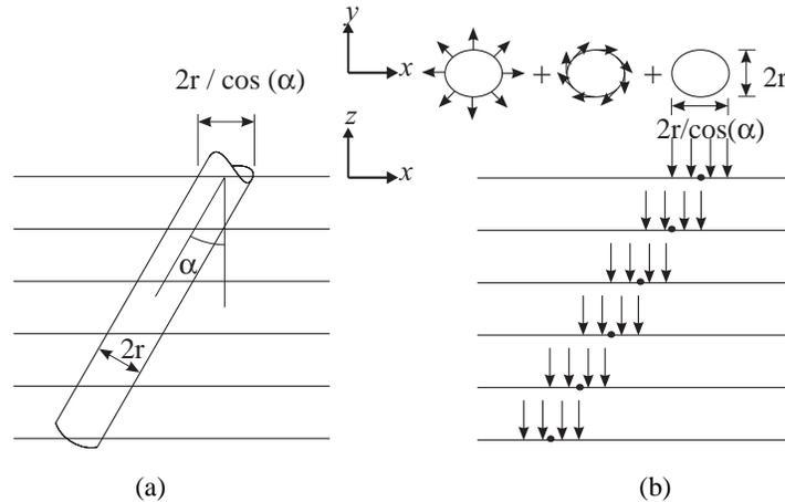
**Figure 1. Inclined pile: a) physical model; b) ellipse-shaped load distributions at the interaction nodes.**
