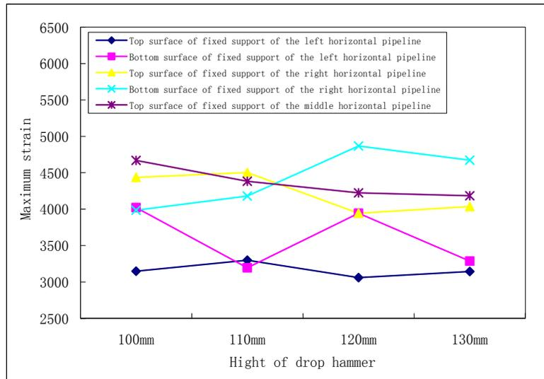
Figure 3.5 Maximum strain under shock on the fixed pipeline segment ( $\mu\varepsilon$ )
