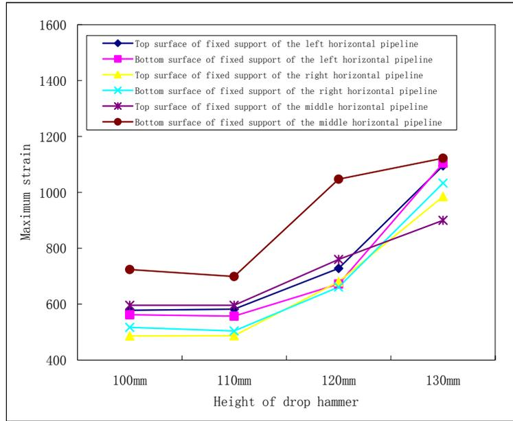
Figure 3.4 Maximum strain under shock on the fixed pipeline segment ( $\mu\varepsilon$ )
