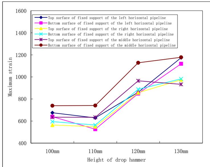
Figure 3.3 Maximum strain under shock on the fixed pipeline segment ( $\mu\epsilon$ )
