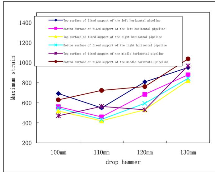
Figure 3.1 Maximum strain under shock on the fixed pipeline segment ( $\mu\epsilon$ )
