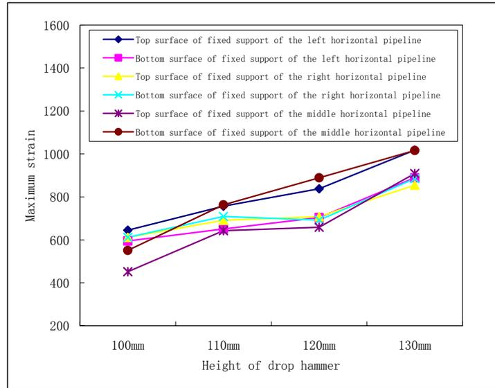
Figure 3.2 Maximum strain under shock on the fixed pipeline segment ( $\mu\epsilon$ )
