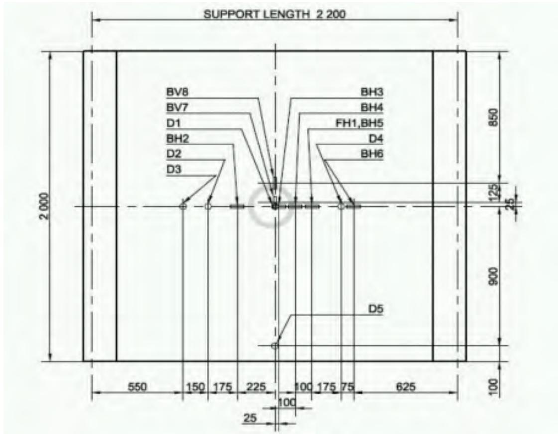
**Fig. 6.** The impact target of the test #643 is the square simply supported reinforced concrete slab of 150 millimeters thickness and with side length of 2.2 meters. There is one way longitudinal reinforcement in the slab with reinforcement ratio of 0.70 %.
