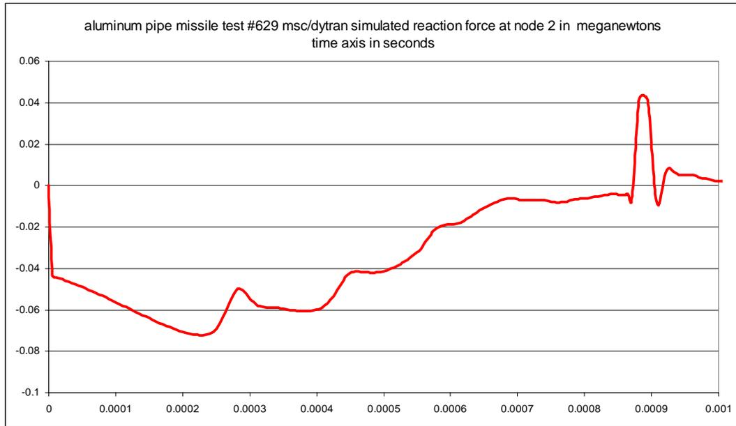
**Fig. 3. Aluminum pipe missile test #629 MSC/DYTRAN simulated reaction force at node 2 in MN:s. Time axis is in seconds**
