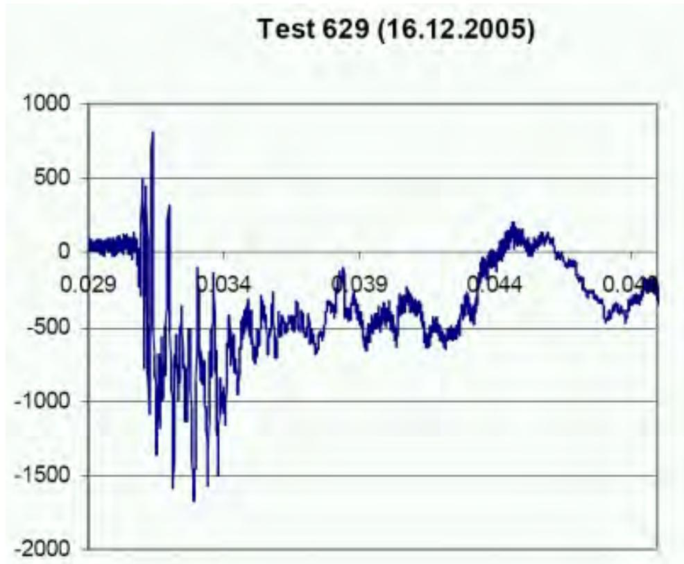
Fig. 4. Aluminum pipe missile test #629. Measured reaction force.
