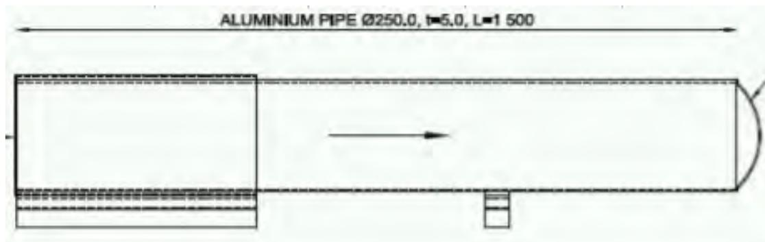
Fig. 5. Schematic presentation of the aluminum projectile used in test #643 at concrete slab target
