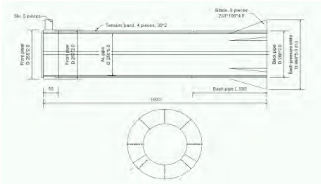
**Fig. 1. Schematic presentation of the aluminum projectile used in simulated test #629.**
