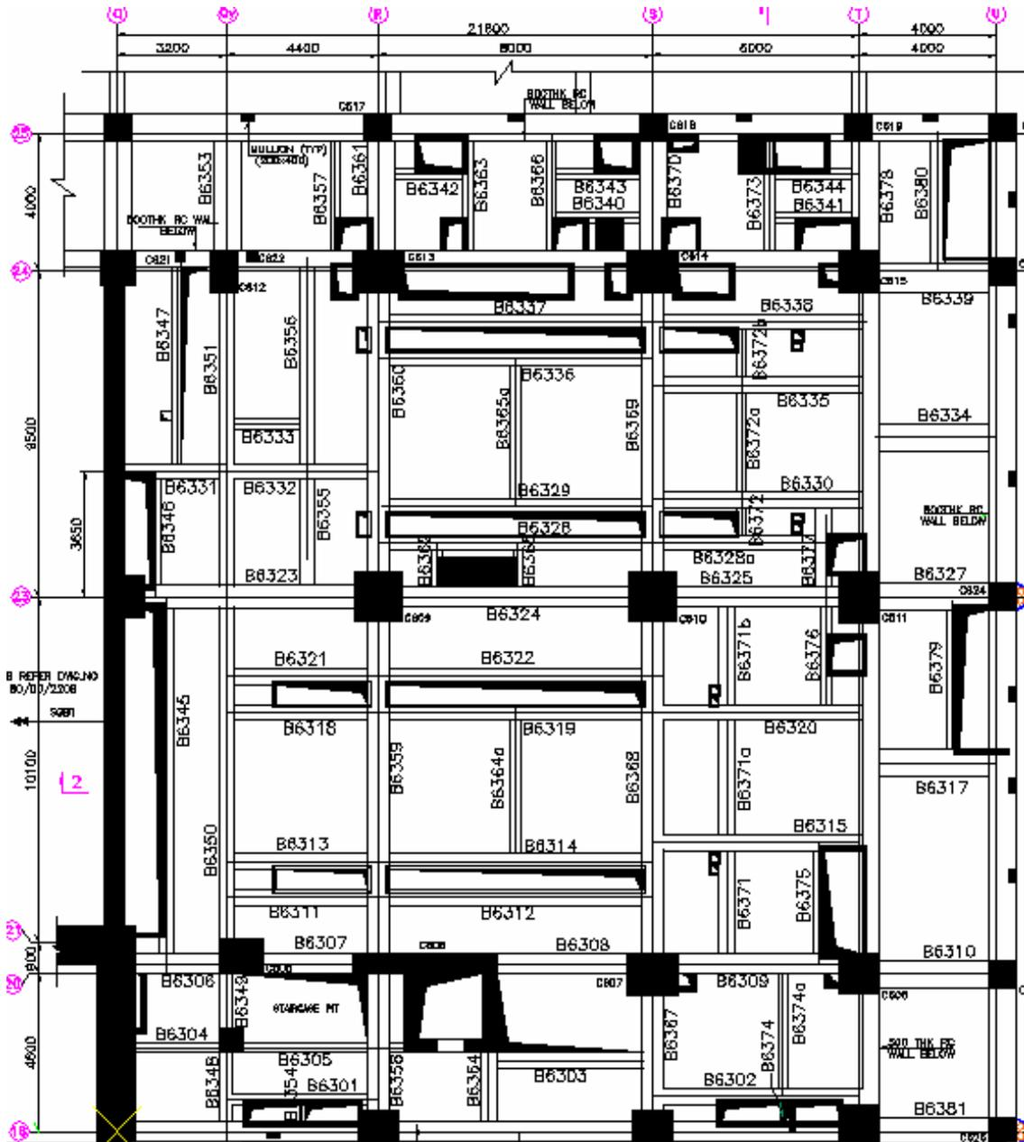
**Figure 5a Layout of Primary and Secondary Beams in EB1 at EL 30000**
