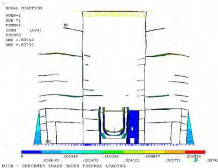
Figure 4: Deformed Profile NICB under Thermal Loads
