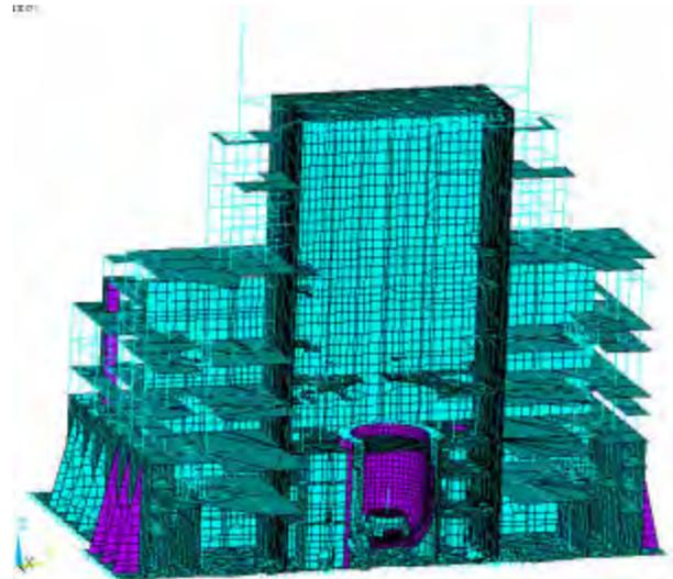
Figure 3: Cross Sectional view of 3-D Model NICB
