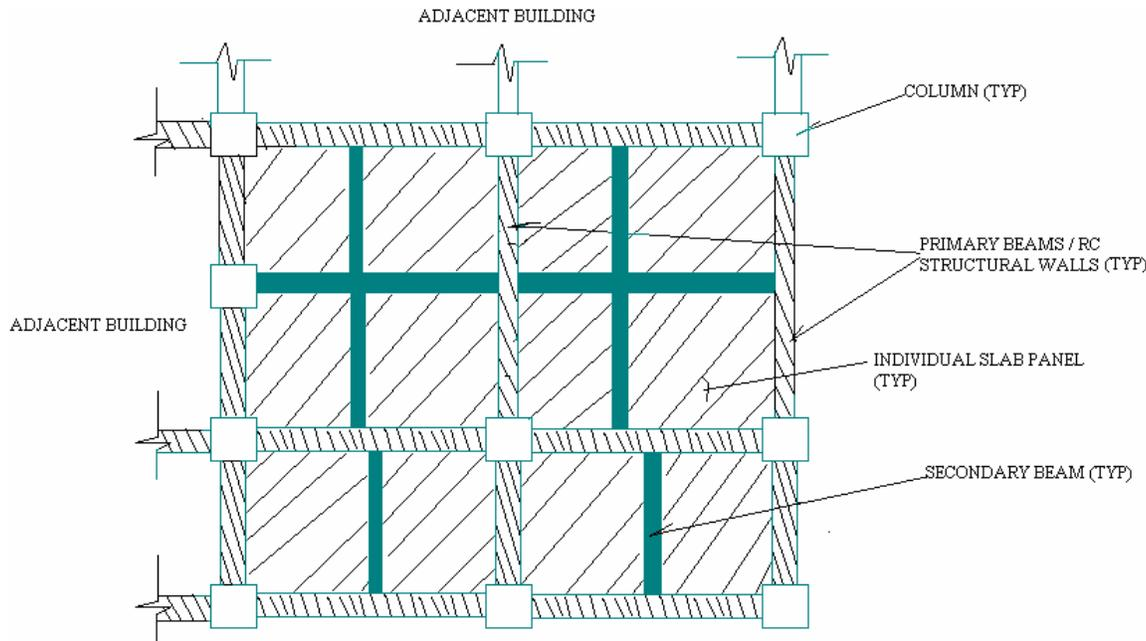
**Figure 1: Layout of a Typical Sub model of Floor, Indicating Primary and Secondary Beams, Slab Panels, Shear Walls and Columns**
