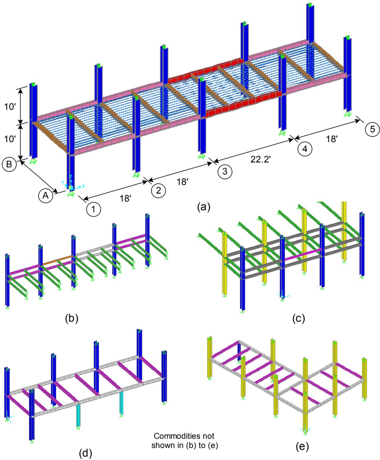
Figure 1: Commodity Rack Configurations
