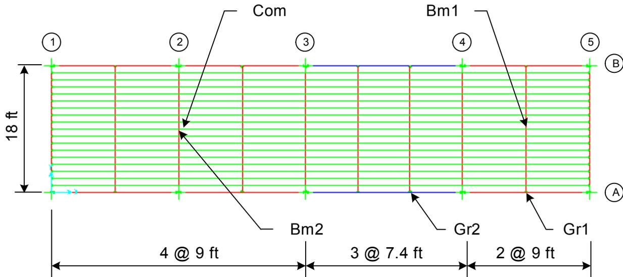
Figure 3: Commodity Support Structure with Selected Moments
