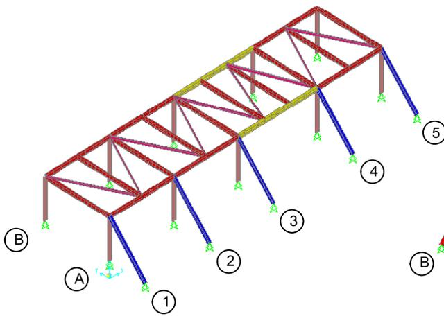
Figure 4: Lateral Braced Rack
