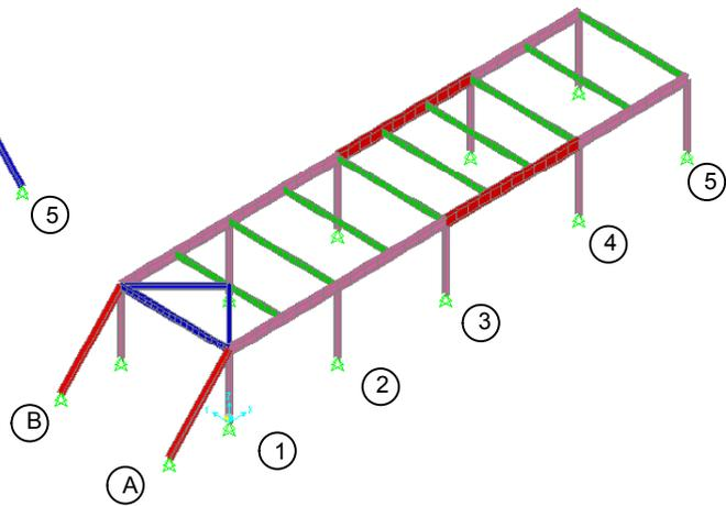
Figure 5: Longitudinal Braced Rack
