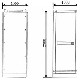
Fig.3-1c Logic Circuit Control Panel
