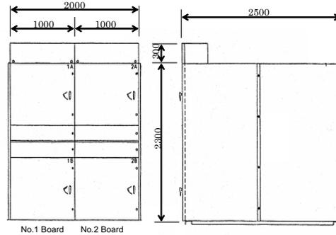
Fig.3-1h 6.9kV Metal-Clad Switchgear
