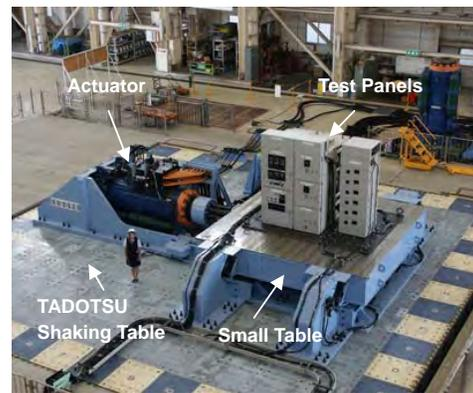
Fig.3-2 Overview of the Test
