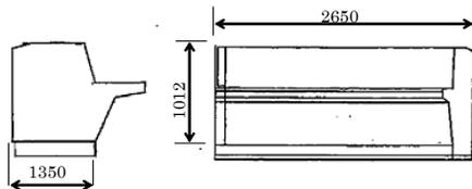
Fig.3-1a Main Control Board
