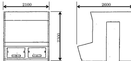
Fig.3-1b Reactor Auxiliary Control Board
