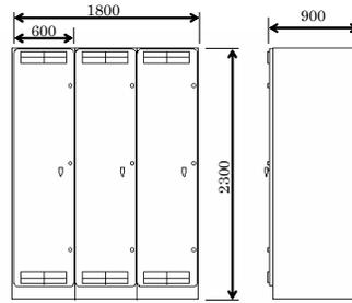
Fig.3-1d Reactor Protection Rack
