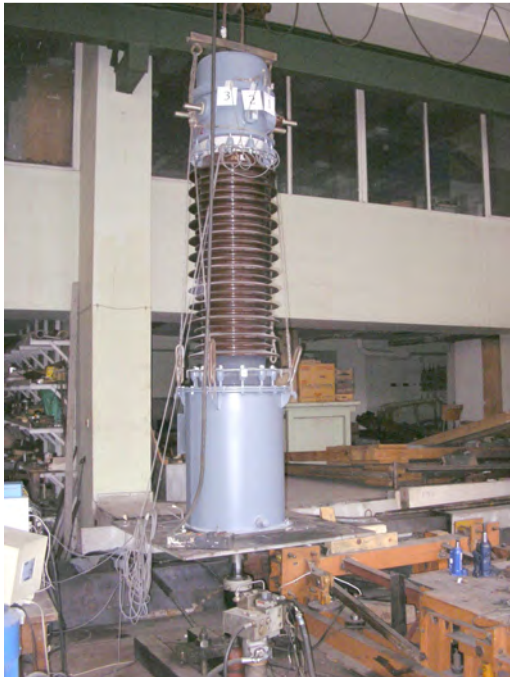
Fig. 6 Testing of current transformers
