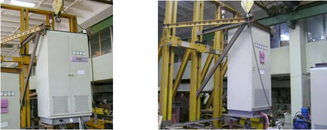
**Figure 3. Pictures of the upgrading structure for the rectifier and inverter testing in vertical direction**
