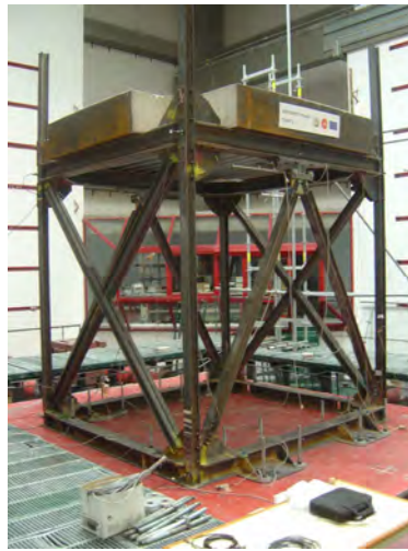
Fig. 1 – Specimen on the LNEC 3D shaking table
