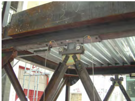
Fig. 2 - View of the Dorka shear panel devices
