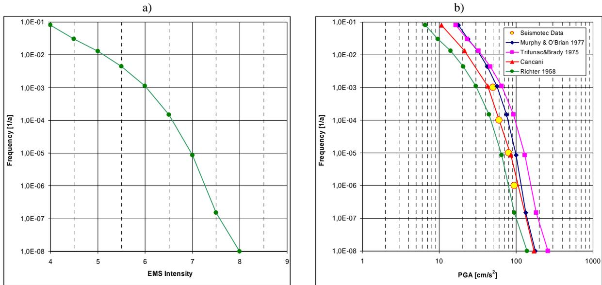
**Fig. 2: Seismic hazard curve for GKN I:**
